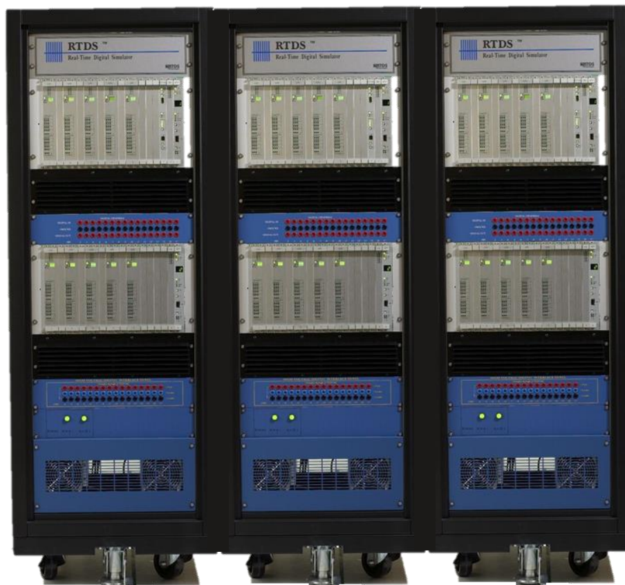
Figure 4 Multiple RTDS racks
