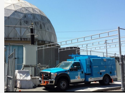
Distributed Gen. Test Yard (DGTY) DER testing up to 2500 kVA
