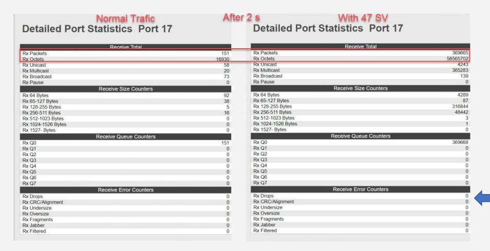
In an Ethernet switch installed in the Process
