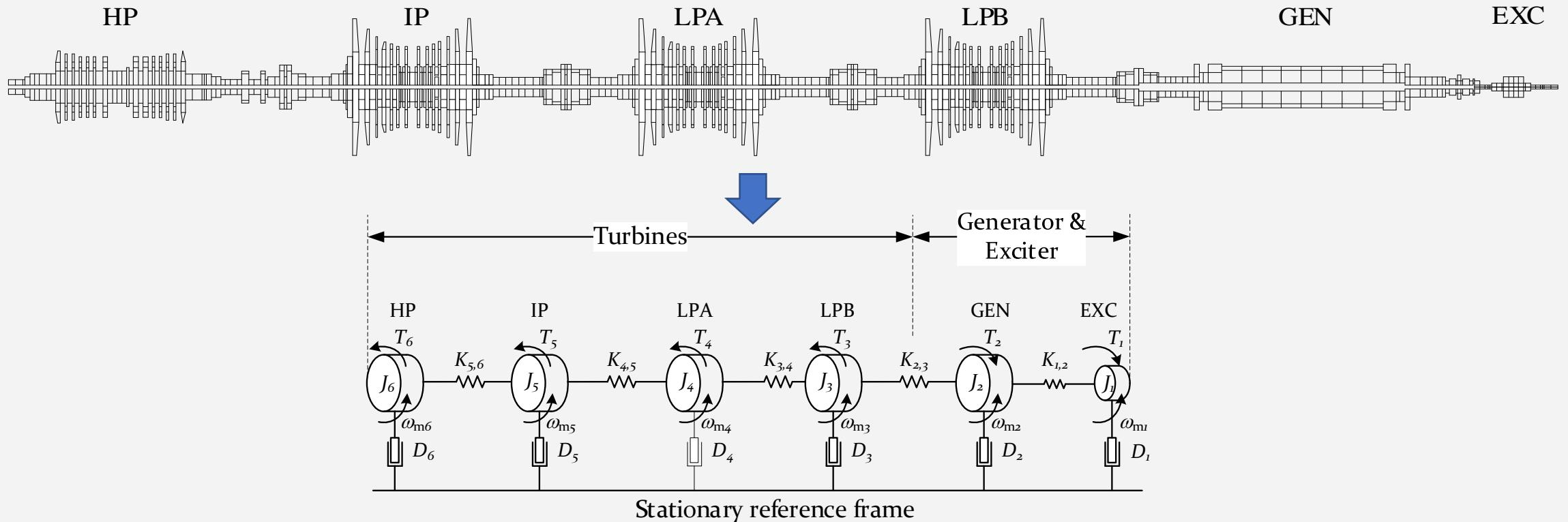
The differential equation describing the dynamic of a mass that is connected by an elastic shaft to its adjacent masses:
