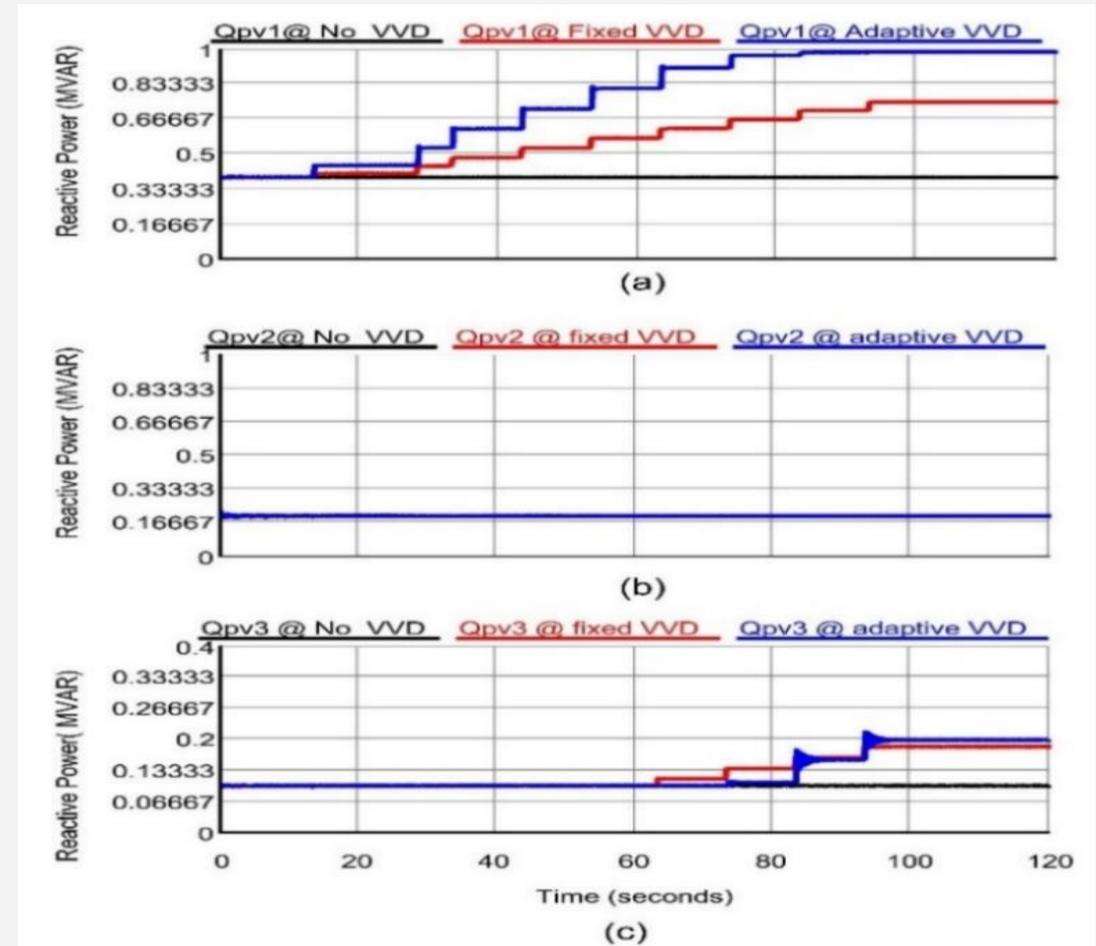
**Fig.2 Reactive power compensation through (a) PV1 (Qpv1) (b) PV2 (Qpv2) (c) PV3 (Qpv3) system under No VVD, fixed VVD and with Adaptive VVD control**
