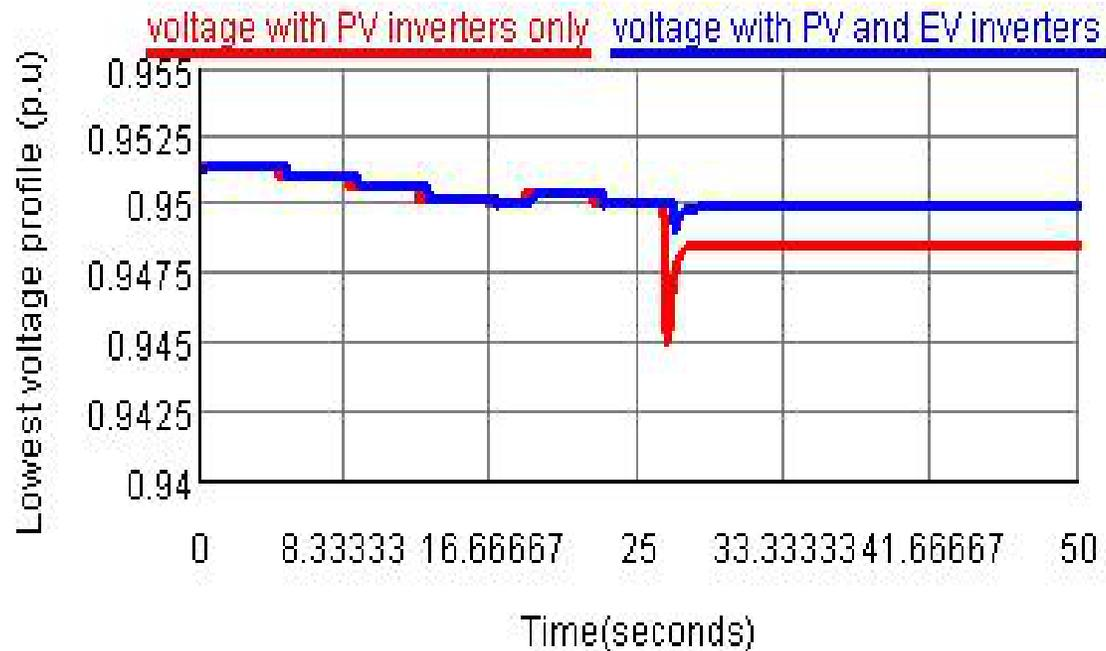
Compensated VAR support from PV2 and EV inverter at node 890
