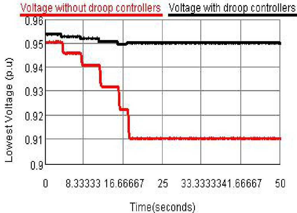
PV Inverter reactive power compensation without and with droop controls
