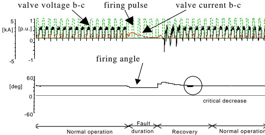
**Fig. 7 Simulation in the Instantaneous Value Mode**
