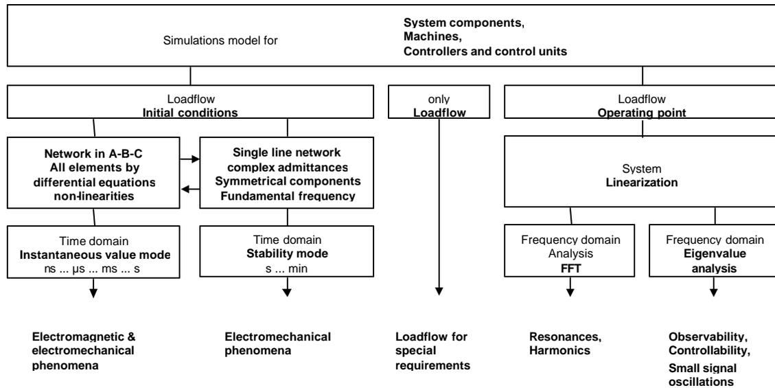
**Fig. 3 Overview of the NETOMAC Simulation Program**
