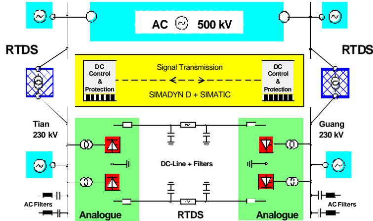
**Fig. 11 Hybrid HVDC Simulator Set-up for the Investigation of Parallel AC/DC Operation**
