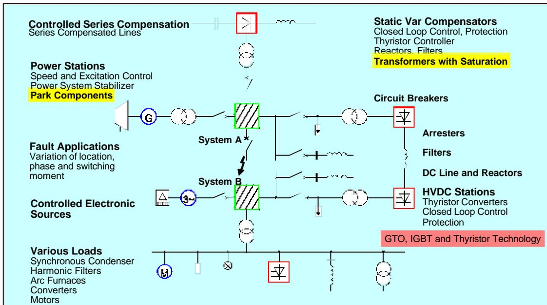
**Fig. 9 Overview of Power System Models for Real-Time Simulation**
