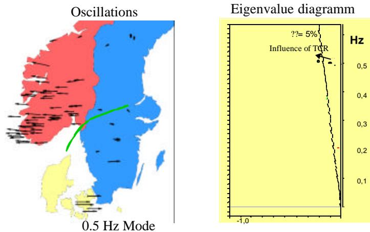
**Fig. 8 Results of “Eigenvalue analysis” in the NORDEL system**
