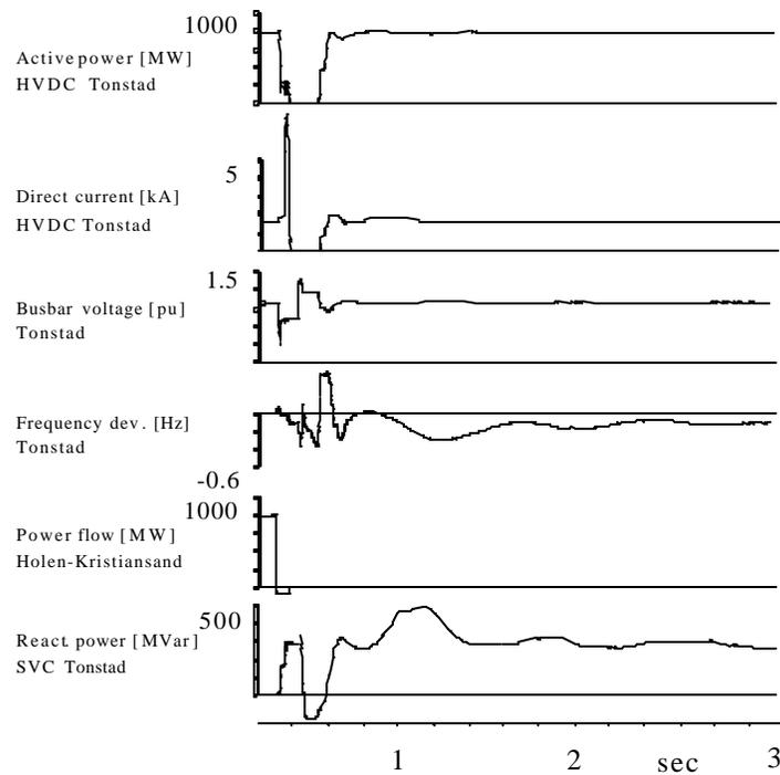
**Fig. 6 Influence of the HVDC Transmission in Tonstad during the Outage of the Line Holen-Kristiansand**
