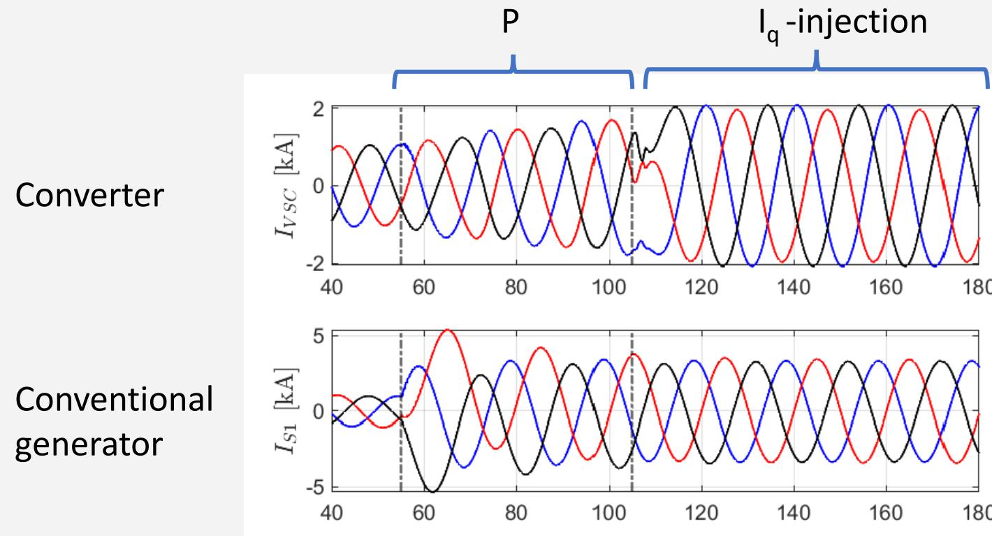
\* Exaggerated delay of fault current injection for purpose visualisation
