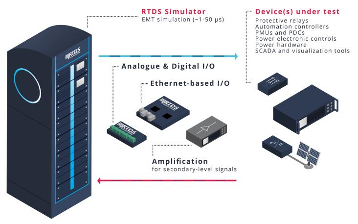
Hardware-in-the-loop testing with the RTDS® Simulator
