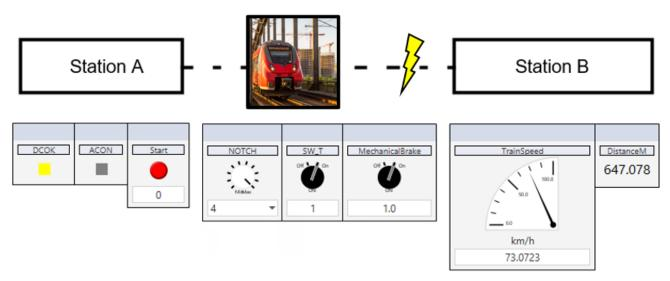
Running a real-time traction simulation in the RSCAD FX operator's console
