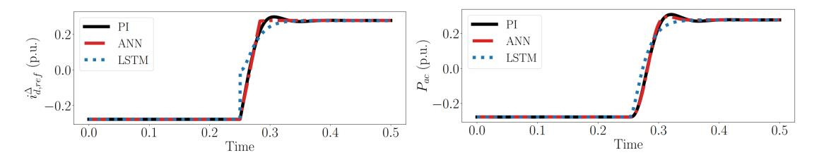
Significantly lower peak overshoot is observed when using an LSTM-based controller
