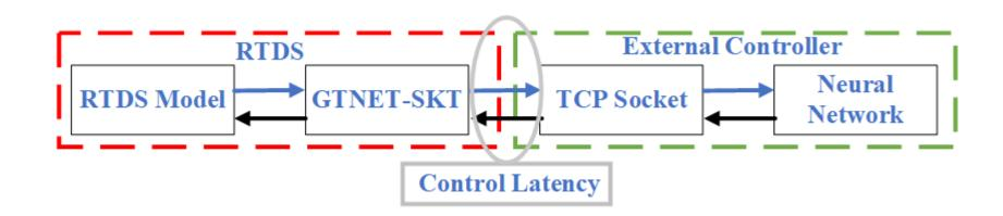
• Significant control latency can hinder the functionality of the controller
