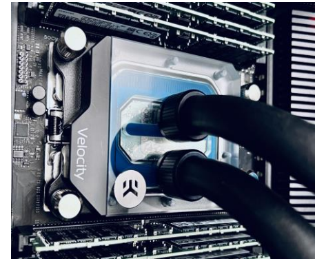
Liquid cooled CPU - AMD Ryzen Threadripper Pro 128 parallel simulations 20hours to run ~500 cases
