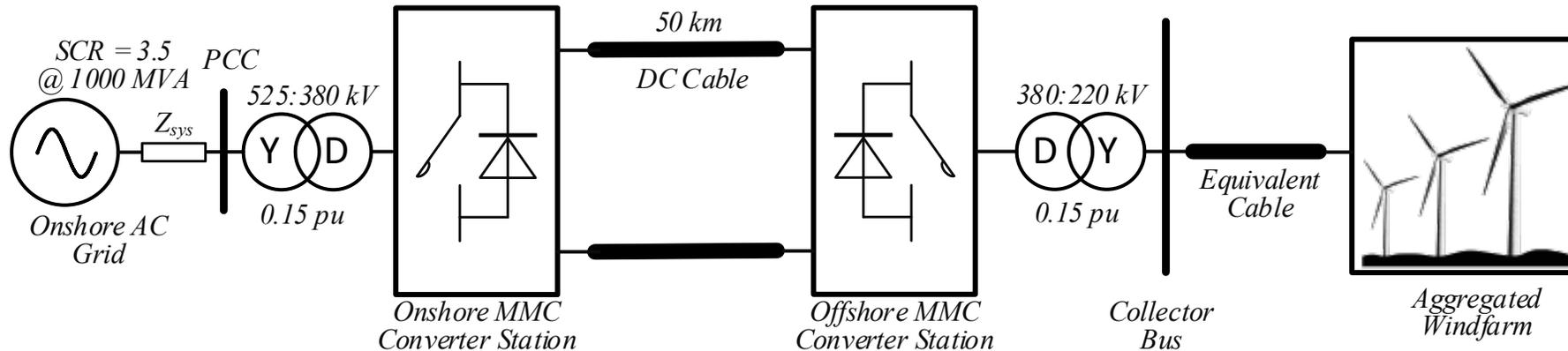
Figure 4-1 MMC-HVDC Offshore Windfarm
