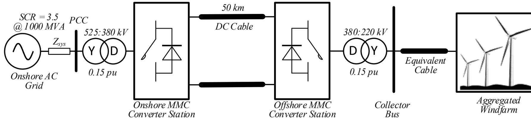
Figure 2-1 MMC-HVDC Offshore Windfarm
