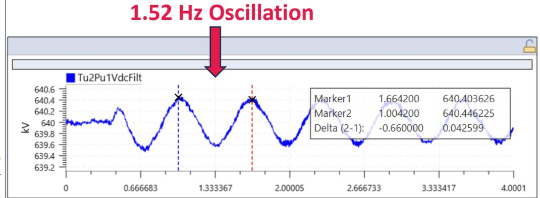
By adjusting the loop gain  $K$  to 0.3425, which means the SCR was adjusted to 1.2, the DC link voltage showed an oscillation frequency of 1.52 Hz at the same operating point. This result matches to what we have observed from the simulation
