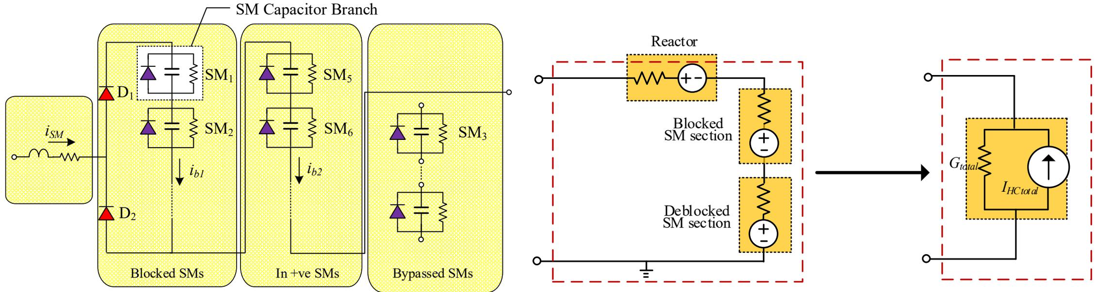
Figure 2-6 Type 4: Detailed Equivalent Model
