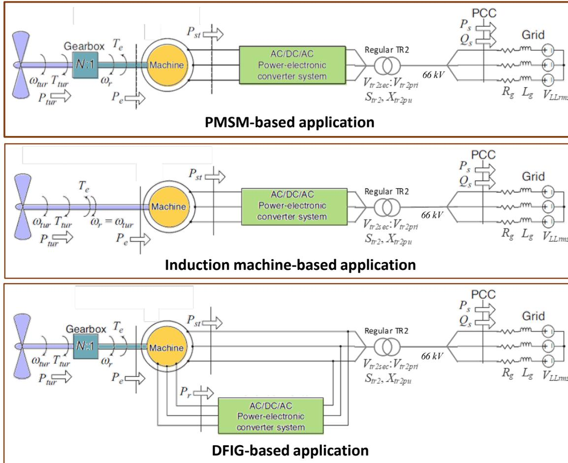
Figure 4-2 Typical Types of Wind Turbine Generators
