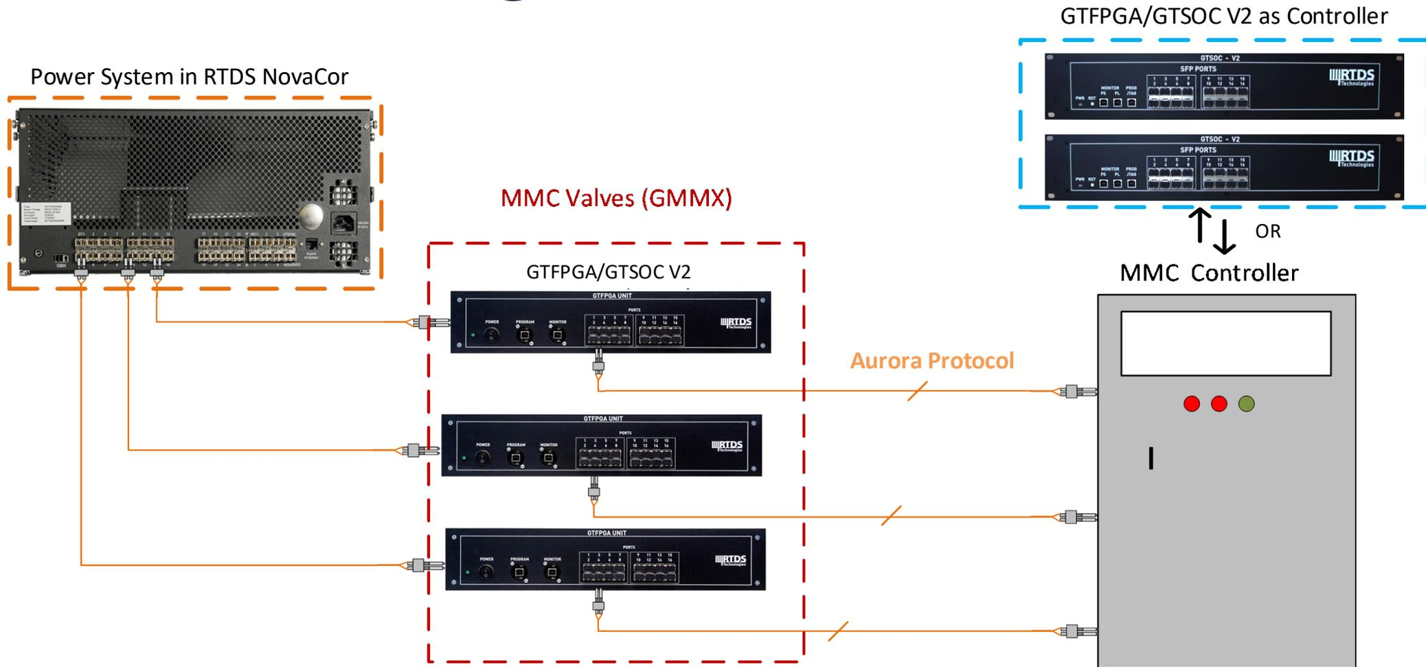
Figure 3-2 MMC CHIL Testing Connection Diagram
