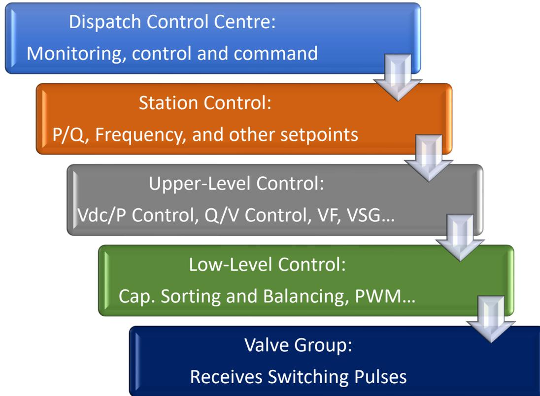
Figure 2-7 Hierarchy Structure of MMC Control [3]
