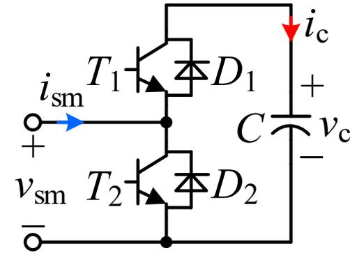
Figure 2-3 Half-bridge Submodule (SM)
