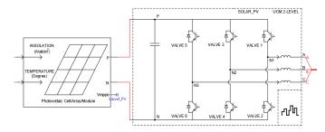
MODEL INVERTER-BASED RESOURCES IN DETAIL. **VENDOR-SPECIFIC BLACK-BOXED CONTROLS** CAN BE INCLUDED IN THE SIMULATION VIA SOFTWARE-IN-THE-LOOP TESTING.
