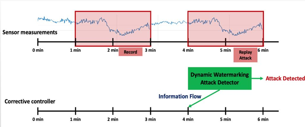
Data Replay Attack through measurement replication.
