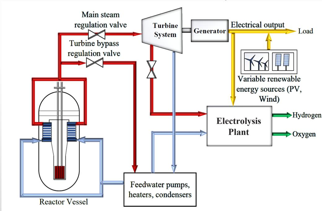
Fig 13: Schematic of SMR for electricity and hydrogen generation
