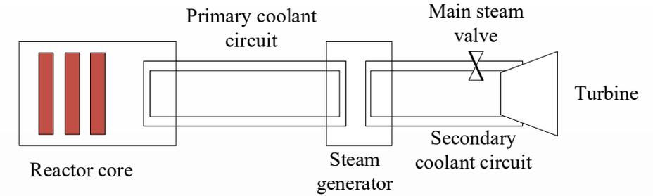
Fig 3: Reactor model components
