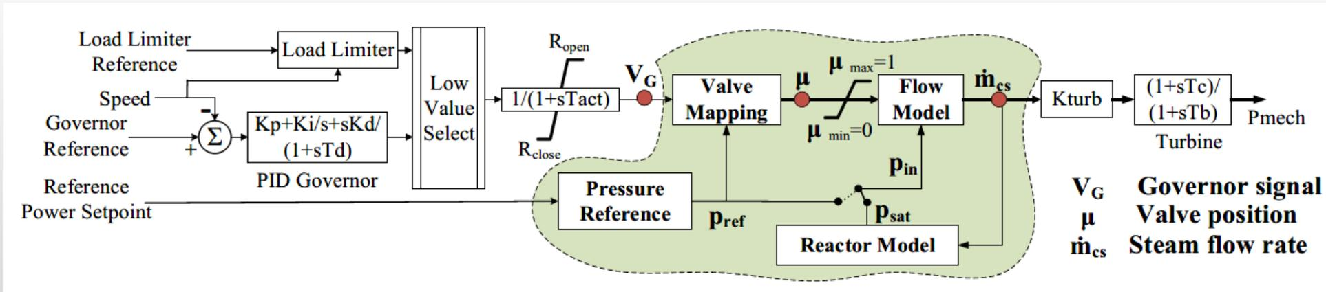
Fig 5: GGOV1 modified and integrated with the SMR model, shaded region shows the modifications with new module
