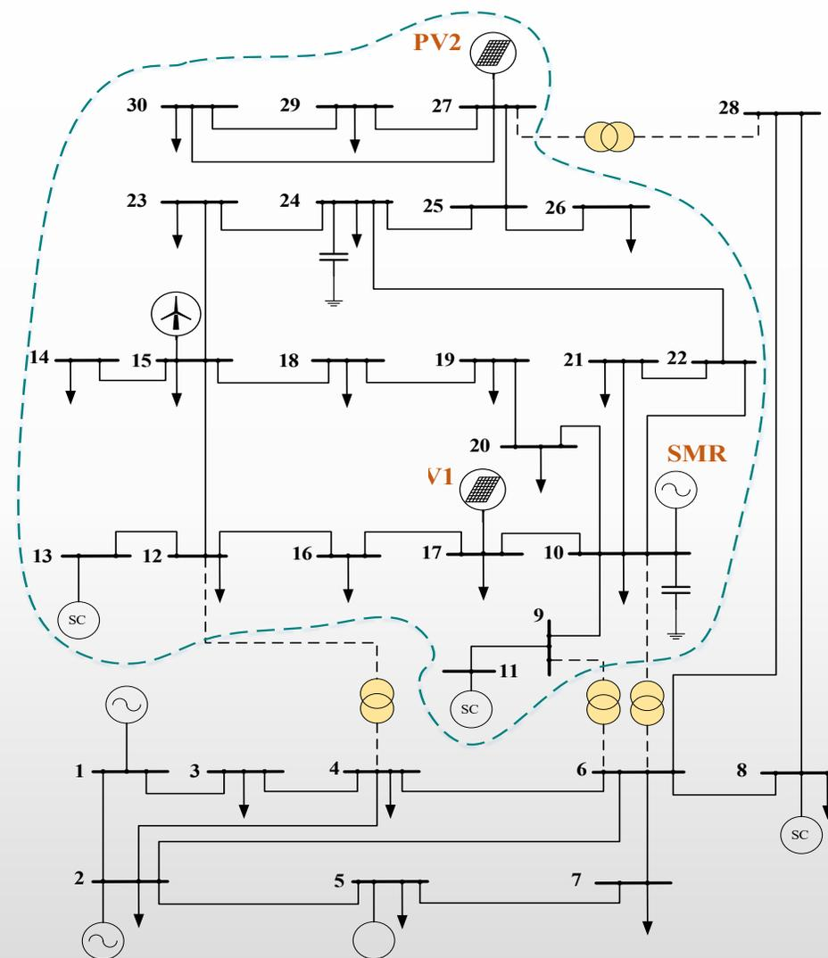
Fig 10: Modified IEEE 30-bus case system
