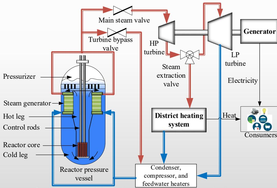
Fig 8: Schematic of SMR for electricity and district heating
