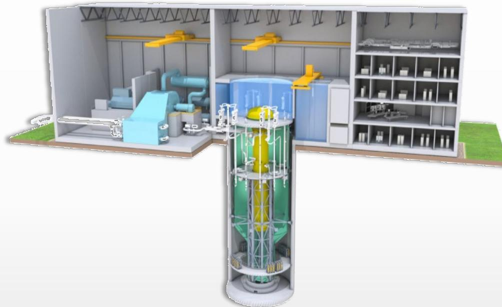
*Fig 1: BWRX-300 small modular reactor*
