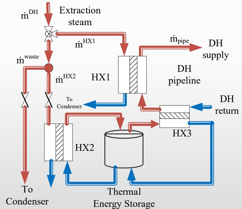
Fig 9: Block diagram of DH system
