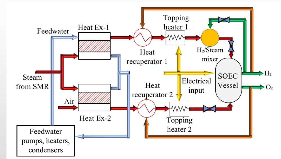
Fig 14: High temperature steam electrolysis for hydrogen generation
