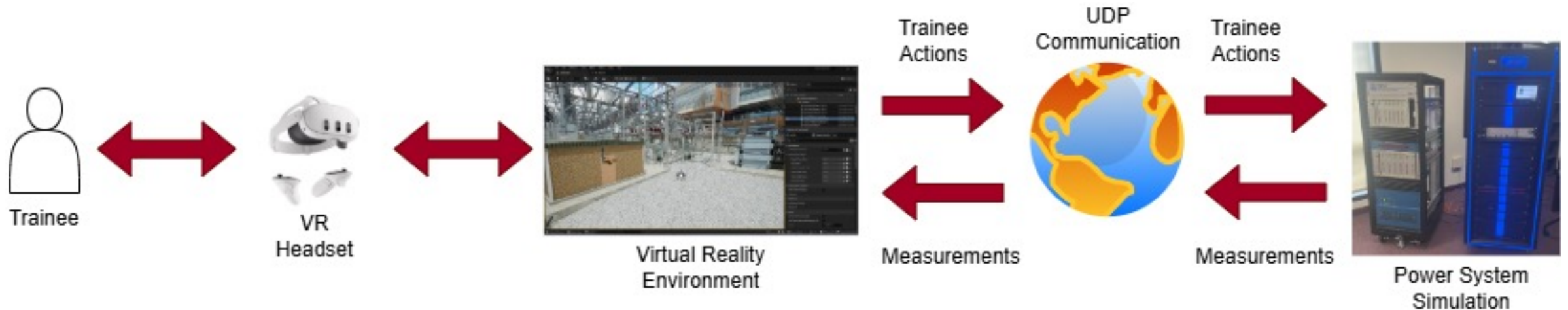
Data flow diagram of the Substation VR project setup
