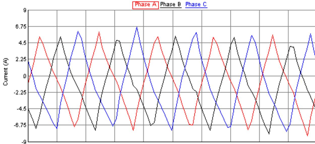
10 kHz ripple current as seen at RTDS. 1 MHz sample rate with 6:1 decimation
