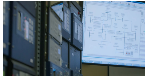
A network simulated with the RTDS ® Simulator is interfaced with SEL relays
