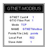
Modbus was introduced in the late 1970s and is used widely today in SCADA and system automation based applications to facilitate communication between a master station and a RTU. It uses the familiar master/slave concept by which the designated master has full control over the communication bus. The master will record outputs and read inputs from each of the slaves who will only respond when requested too by the master.
