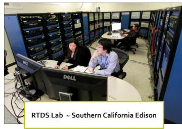
capability so that external control and protection equipment may be interfaced to the simulator for closed loop testing. In addition to traditional analog and digital interface signals, the RTDS also includes LAN based communication protocols for interconnection with IEC capable protective
