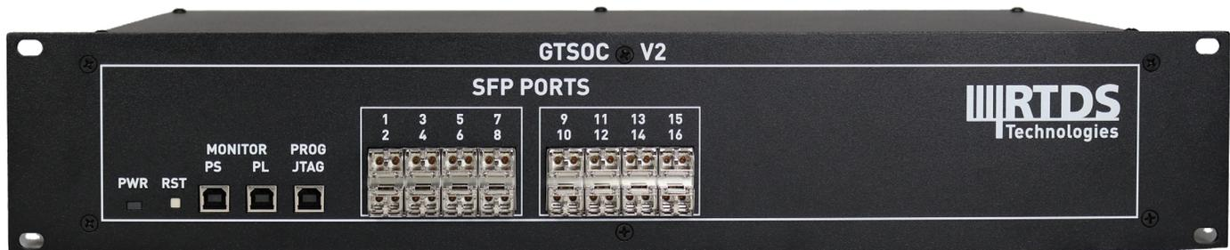
The GTSOC V2 is a multi-function, FPGA-based auxiliary hardware that can be used to represent MMC valves and controls.
