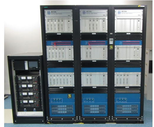
THE RTDS SIMULATOR SETUP AT J-POWER
