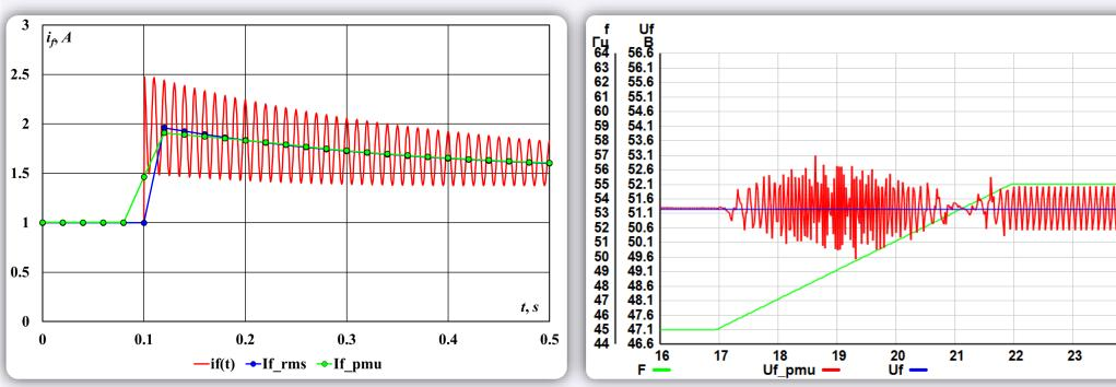
Generator stator short current modelling. Checking filtering  $2 \cdot f_{generator\_base}$ The result signal contains aperiodic component, periodic component with  $2 \cdot f_{generator\_base}$ frequency, step changing component Linear changing of power AC voltage Appearance of pulsating error in measurement result while measurement-window is not equal period of the signal
