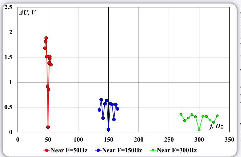
Modeling steady-state work of excitation system after breakdown in the power system. Different values of frequency's near base values (50, 150, 300 Hz).
