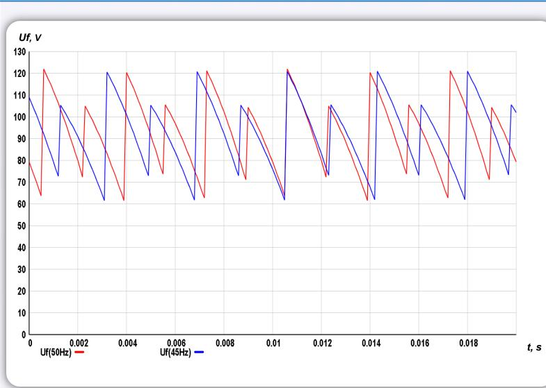
Modeling steady-state work of excitation system after breakdown in the power system. Different values of frequency's near base values (50, 150, 300 Hz).
