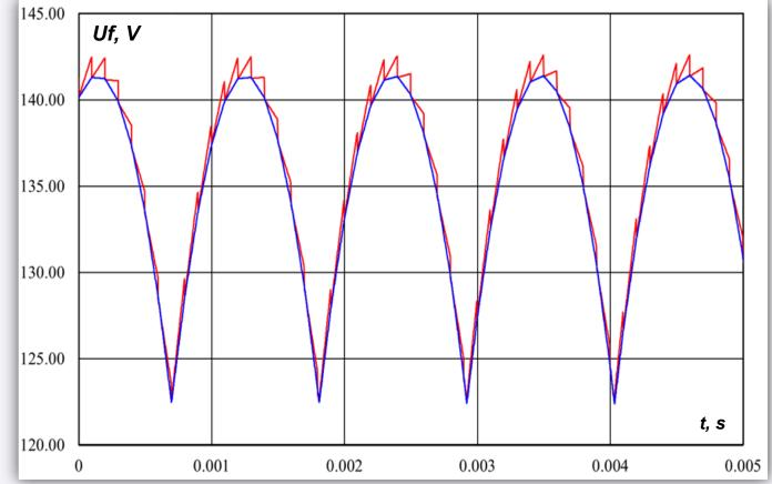
$u_{f}(t, f_{AC}=150 \text{ Hz})$  large-dt,  $u_{f}(t, f_{AC}=150 \text{ Hz})$  large-dt+small-dt Example of measured voltage amplifier output. **Standard** method (large-dt) and **applied** method
