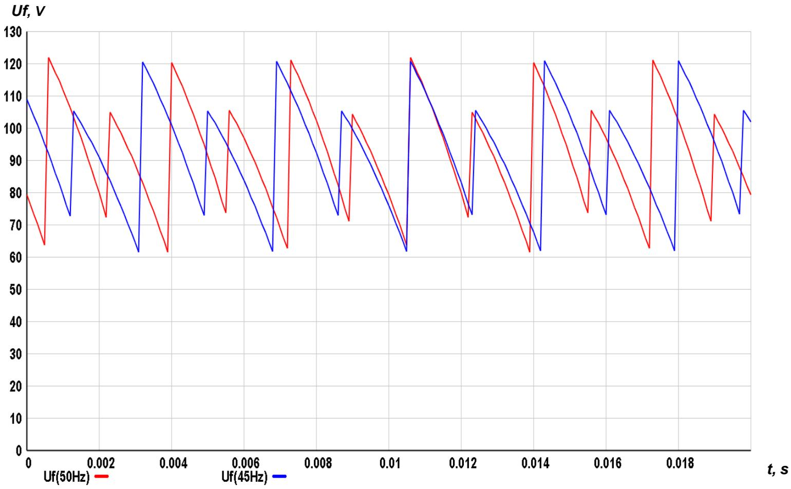
Modeling steady-state work of excitation system after breakdown in the power system.
