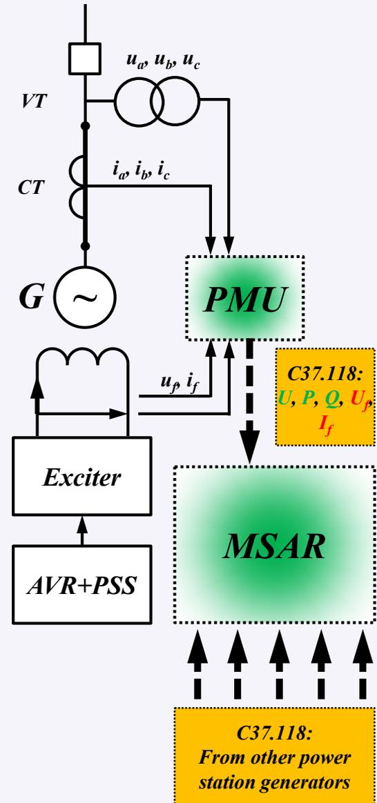
PMUs in Russia should be tested with the special procedure, which was developed on the basis of Standard C37.118. So measurements of  $U, I, P, Q$  are considered correct. Procedure has not requirements for PMU excitation signals measurement. Without this requirements measured  $U_f$  and  $I_f$  can cause wrong conclusions of MSAR algorithm.
