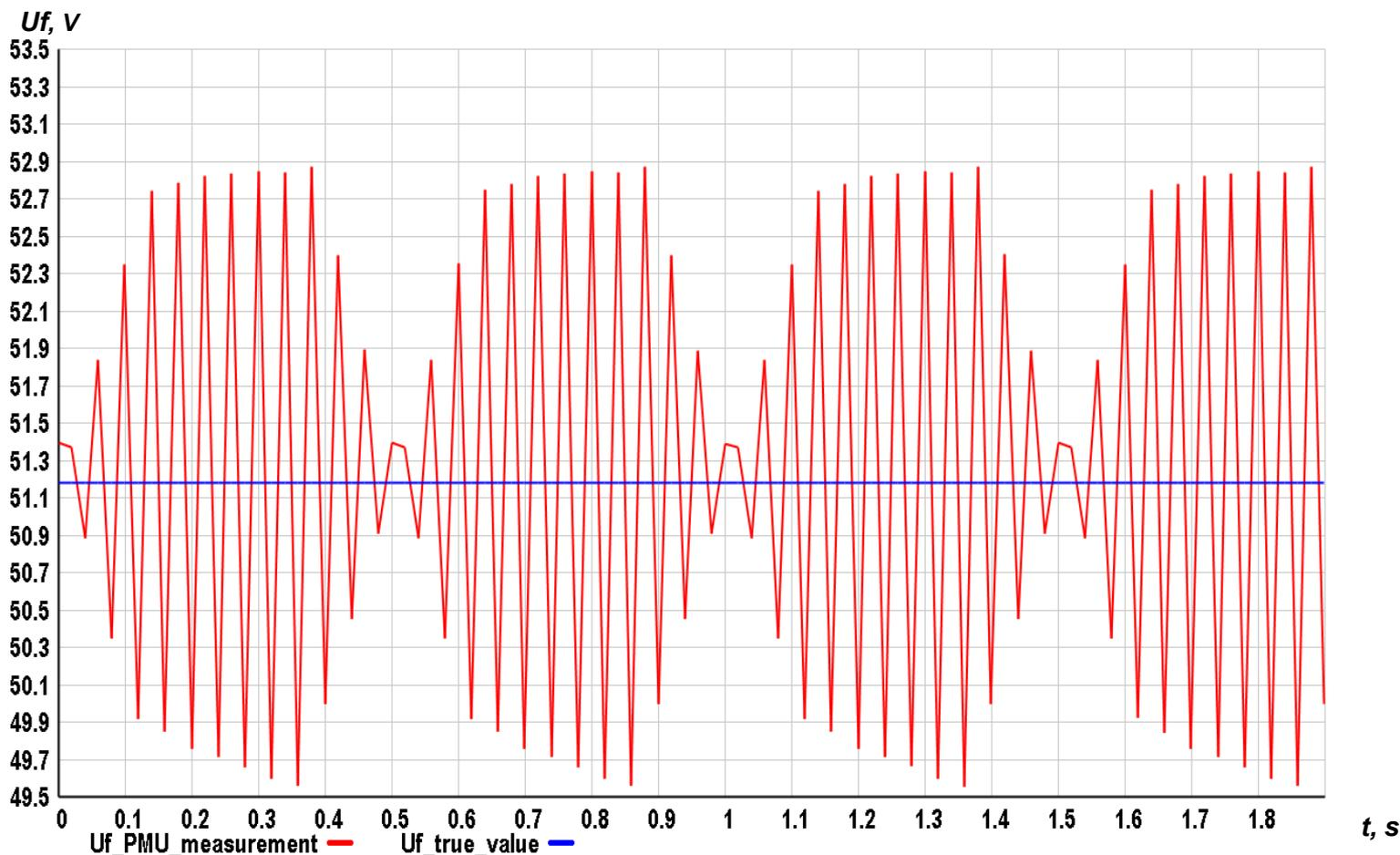
Modelling steady-state work of excitation system after breakdown in the power system.
