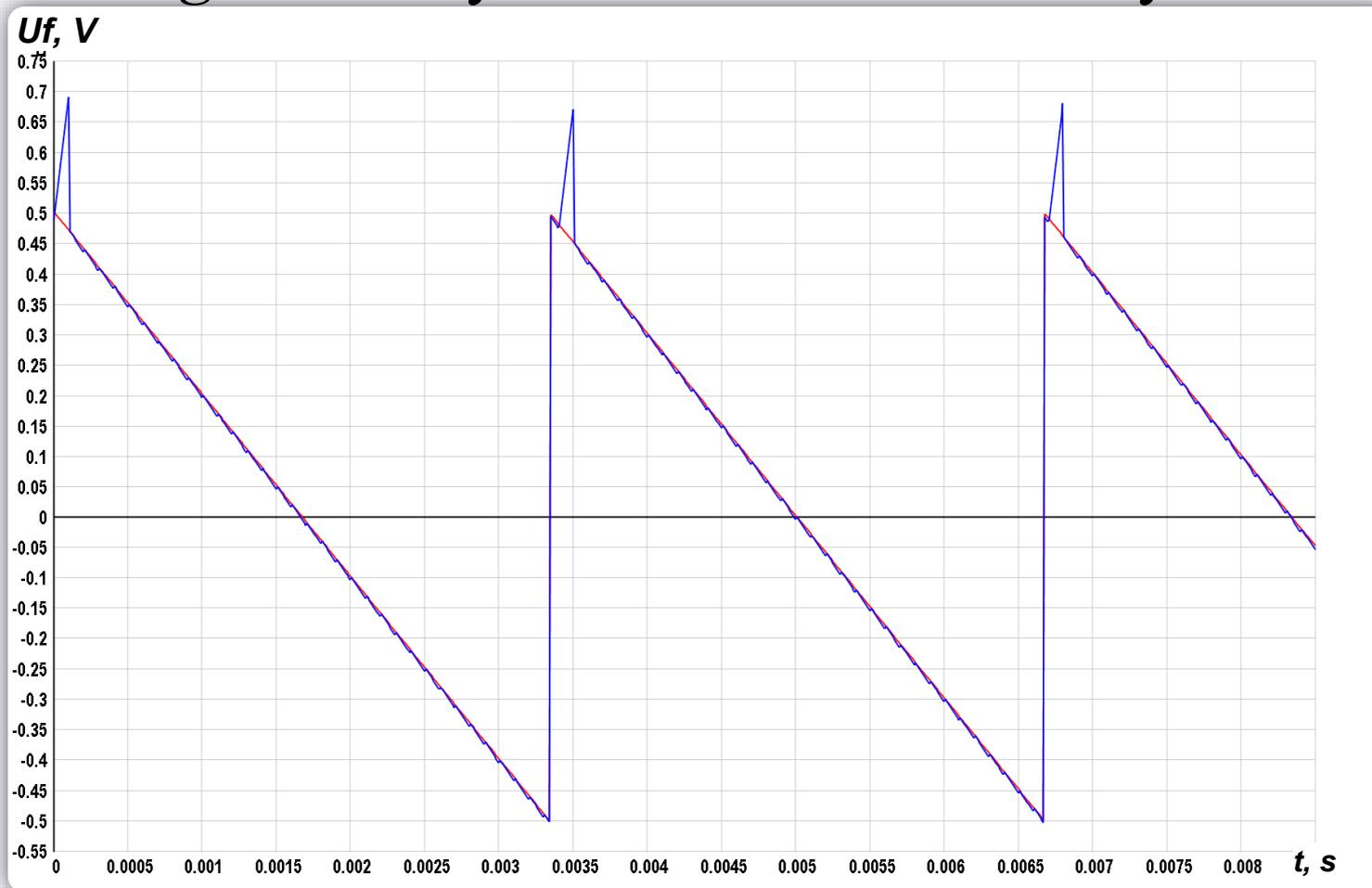
Example of measured voltage GTA0 output.
