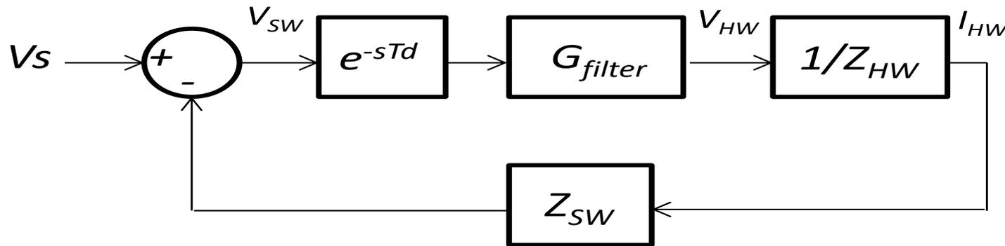
$$G_{OL}(s) = \frac{Z_{SW}(s)}{Z_{HW}(s)} e^{-sTd} \cdot G_{filter}(s)$$
