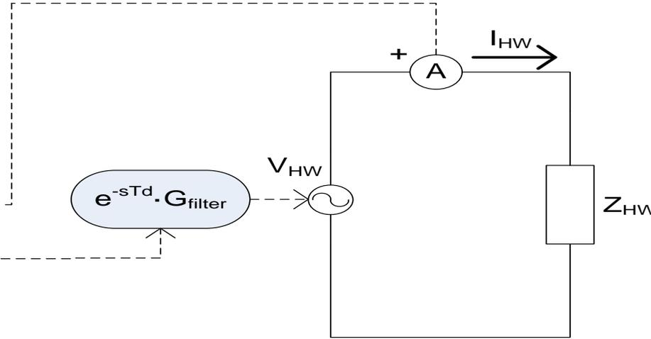
$$V_{HW} = V_{SW} \cdot e^{-sTd} \cdot G_{filter}$$
