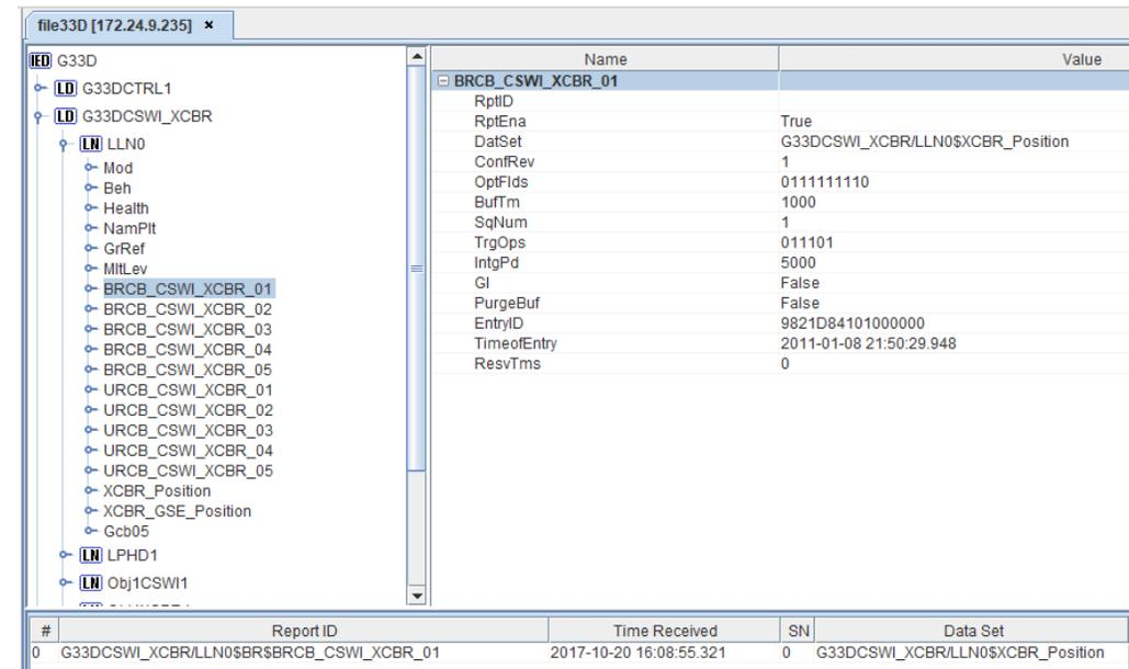
The screenshot shows a software interface for an MMS client. On the left, a tree view displays the hierarchy of logical nodes (LD, LN) under the G33D instance. The selected node is BRCB\_CSWI\_XCBR\_01. On the right, a table displays the values for this node's attributes.
