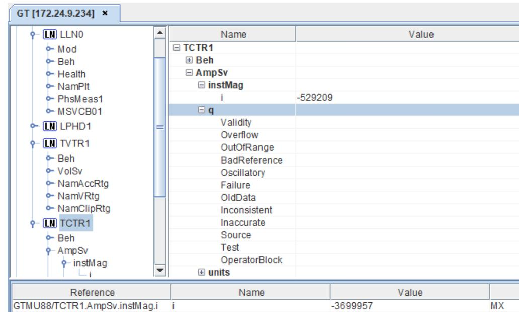
The screenshot shows the GTNETx2-SV v6 MMS client interface. The title bar indicates the connection to GT [172.24.9.234]. The left pane displays a tree view of logical nodes (LN) under the root node LLN0. The selected node is LN TCTR1, which is expanded to show its sub-nodes: Beh, AmpSv, and instMag. The right pane displays a table of data for the selected node, with columns for Name and Value. The table shows the following data:
