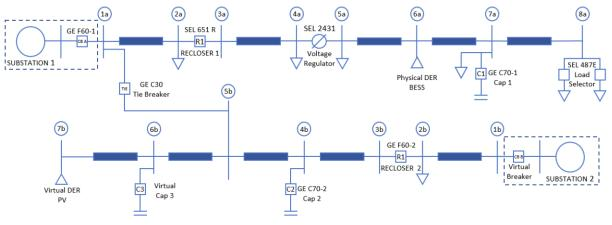
Entire distribution automation schemes including capacitor bank control, bay automation control, feeder protection, recloser control, voltage regulator control, and other components can be connected to a simulated feeder in a closed loop. The interoperability of devices of multiple vendors and functions in a huge variety of contingency conditions can be validated prior to deployment. A combination of virtual and physical assets can be used depending on hardware availability.
