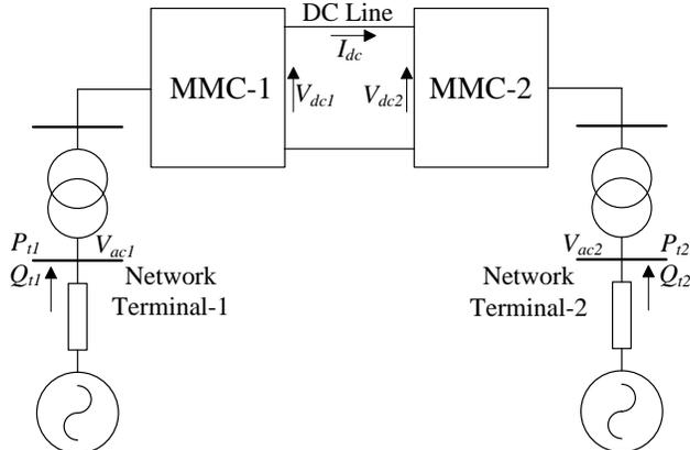
Fig. 1. A point-to-point MMC-VSC system with AC network connections
