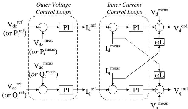
Fig. 2. d-q decoupled control system (ref-reference, meas-measured, ord-order)
