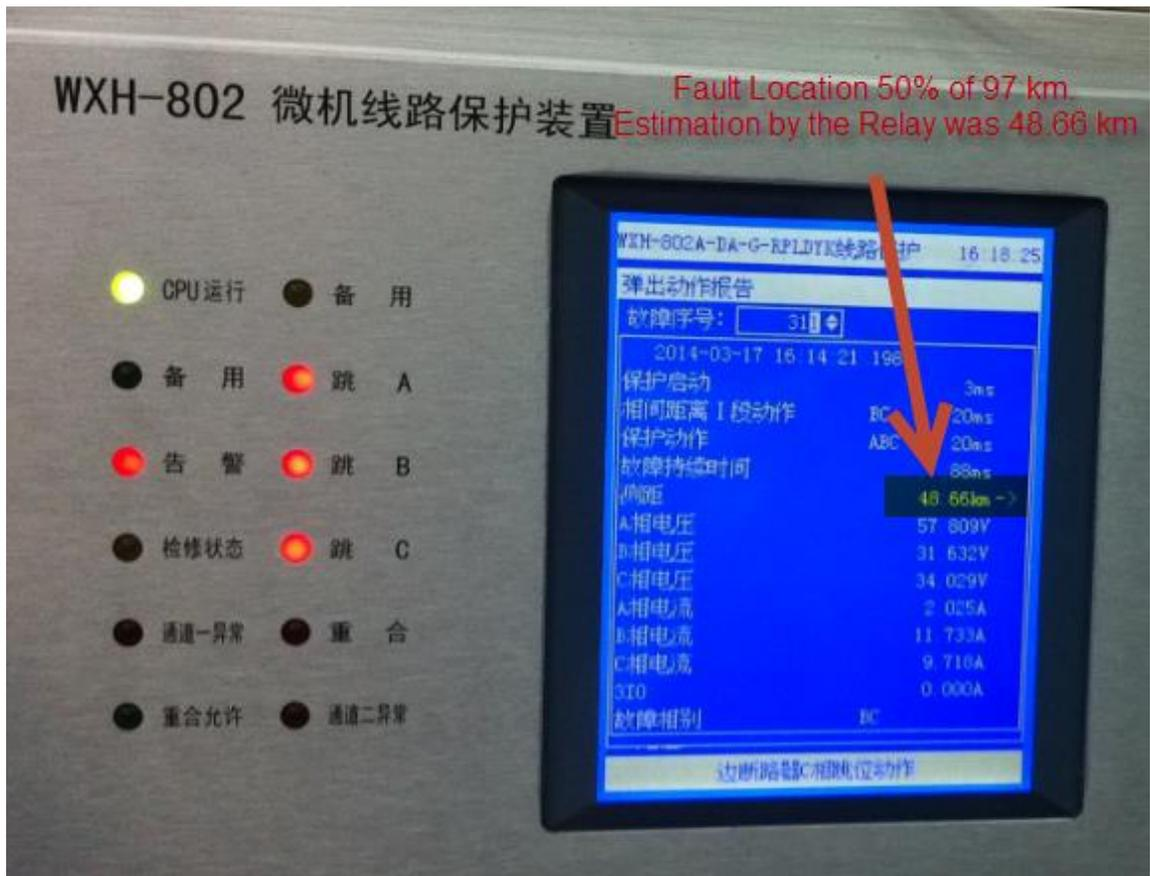
Figure 6: Line Protection Tests Result for fault at 50% of line
