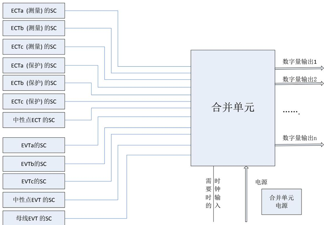
Figure 3 shows a typical configuration of a Chinese merging unit and system architecture of the electric transducer. Note that is typical channel input layout, the channel input layout might be different.
