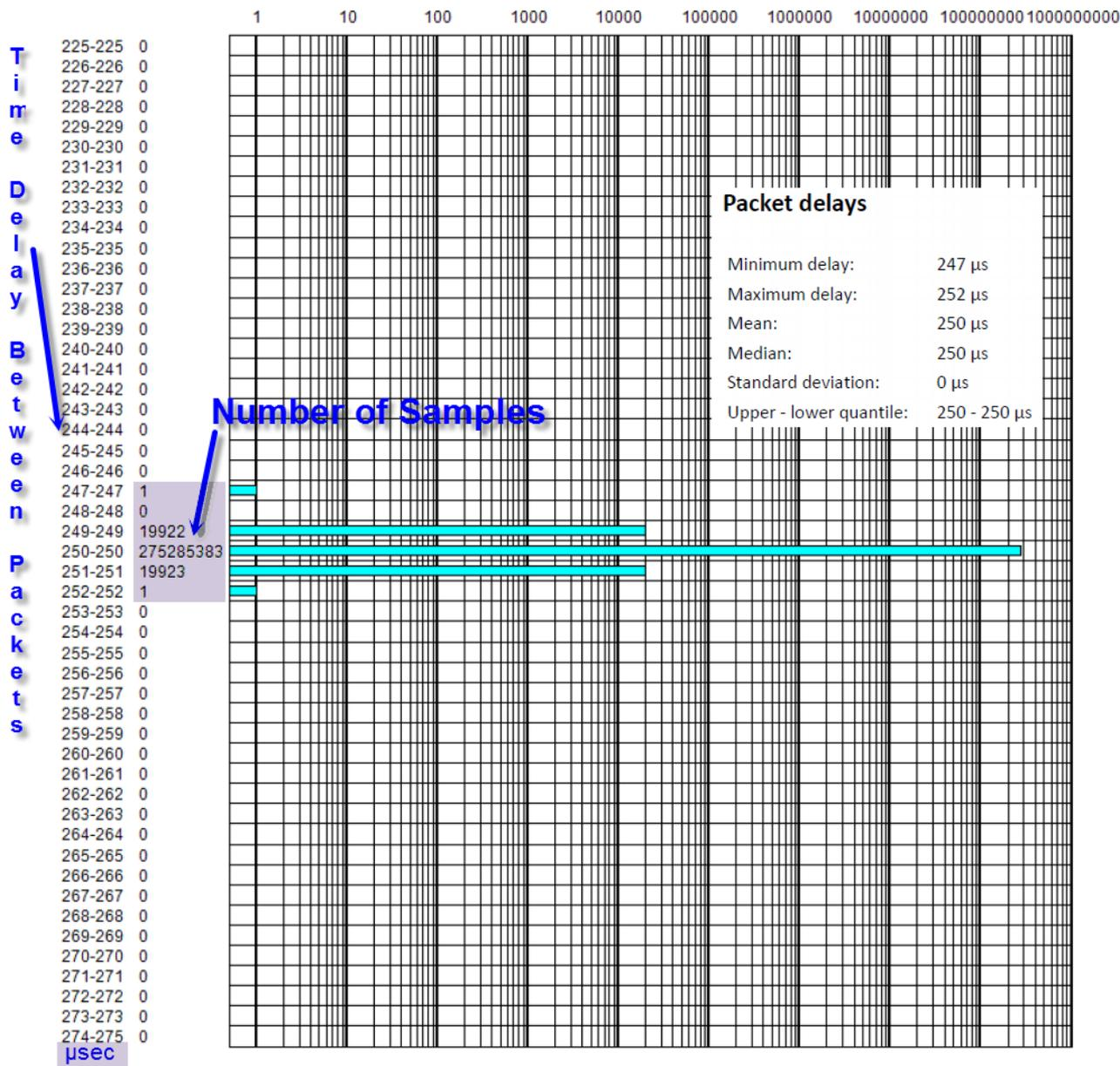
Figure 1: Packet Delay in  $\mu\text{sec}$  from GTNET-SV
