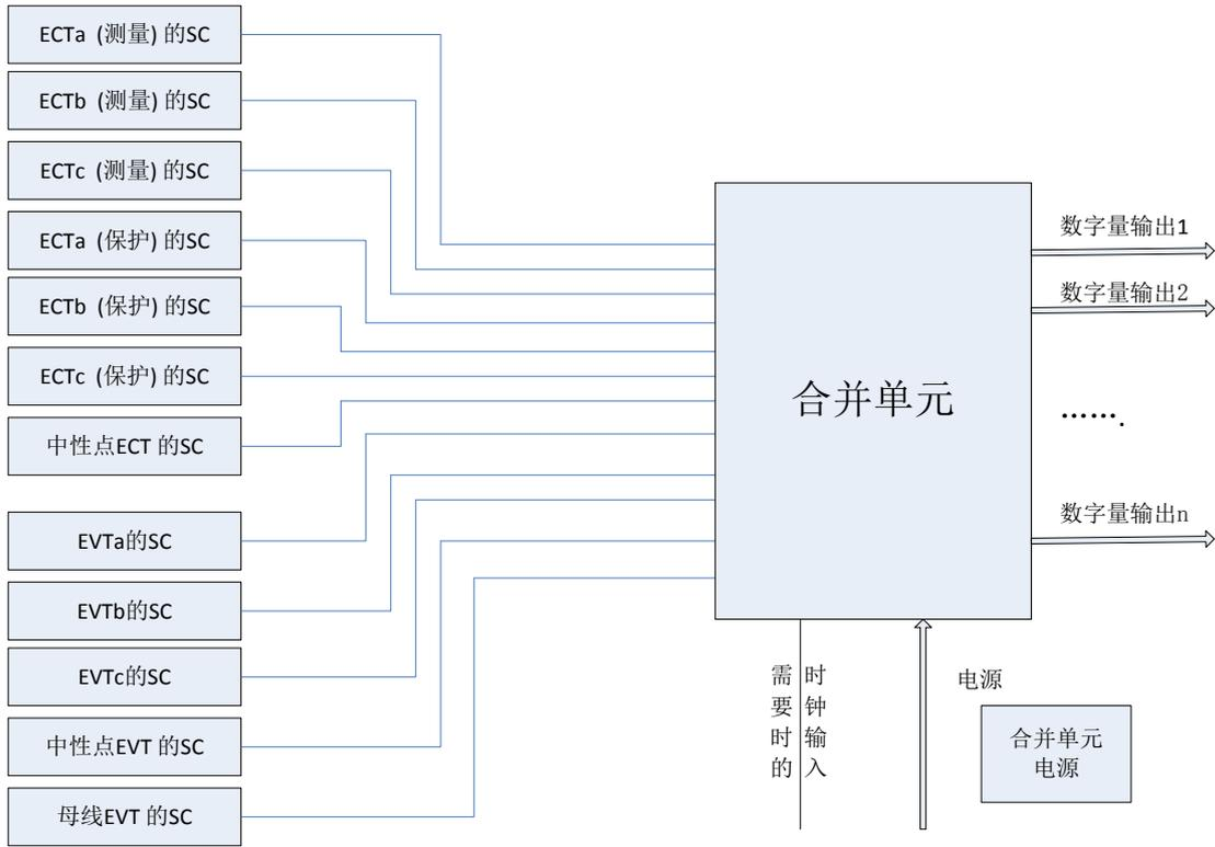
Figure 3: Typical Configuration of Chinese MU
