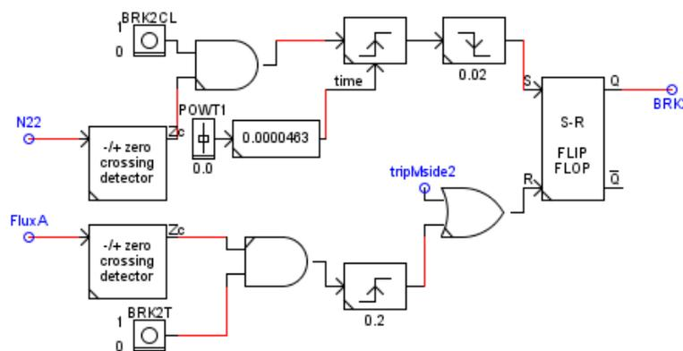
Figure 8: Control Logic to Trap Flux
