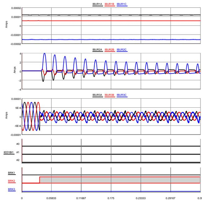
Figure 10: Transformer Inrush Current
