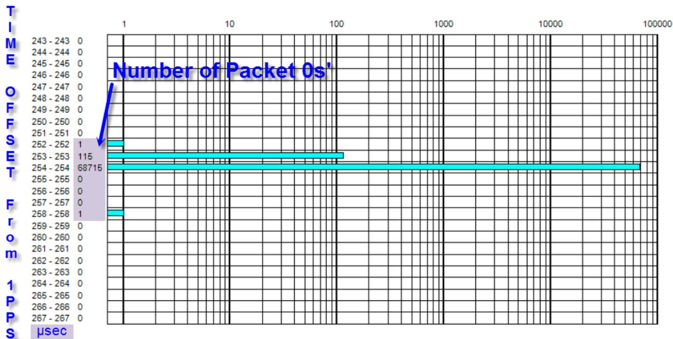
Figure 2: Time Offset from 1PPS in μsec from GTNET-SV
