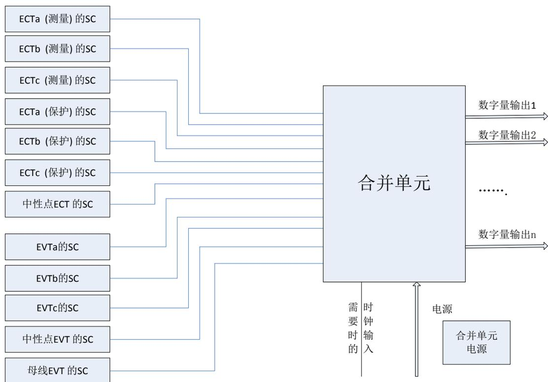
Figure 3: Typical Configuration of Chinese MU
