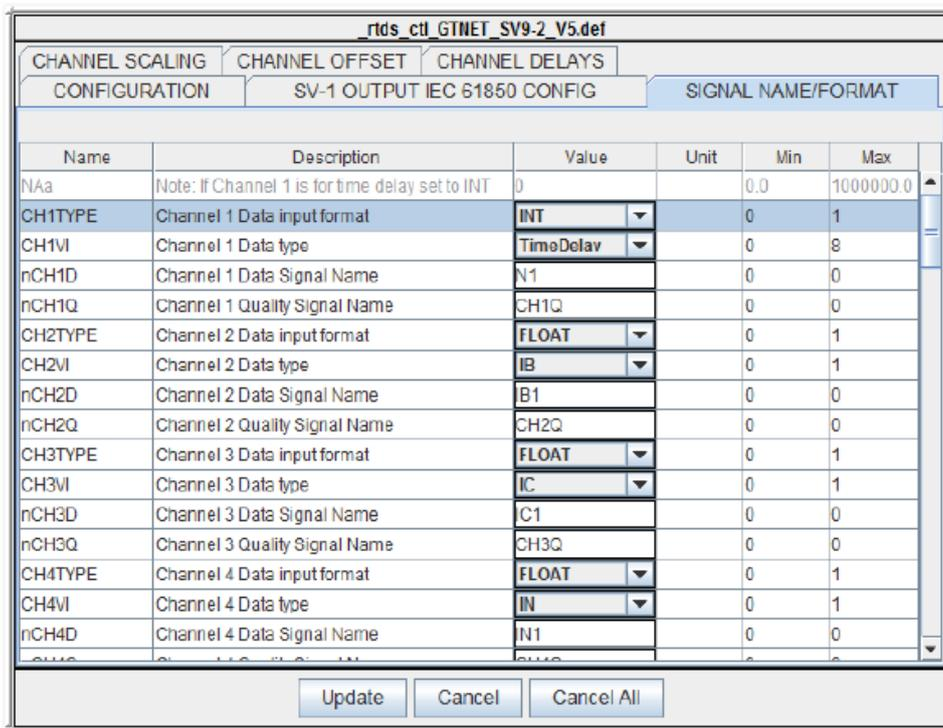
Figure 4: Configuration of GTNET-SV
