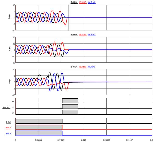
Figure 9: Internal A-N fault and IED operation
