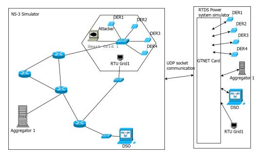
In the graphic on the left, a network simulator is connected to the RTDS Simulator via realtime UDP socket communication.
