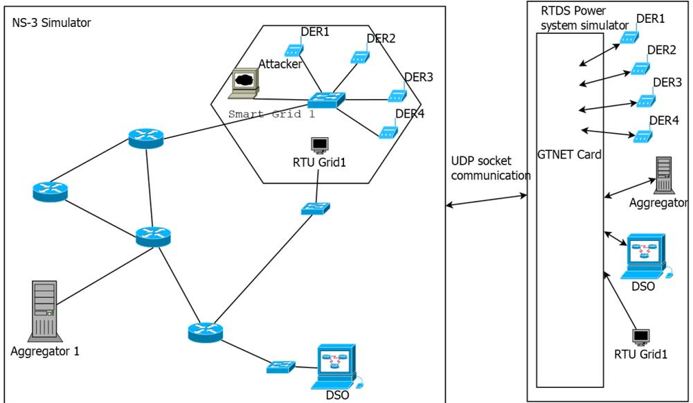
In the graphic on the left, a network simulator is connected to the RTDS Simulator via real-time UDP socket communication.
