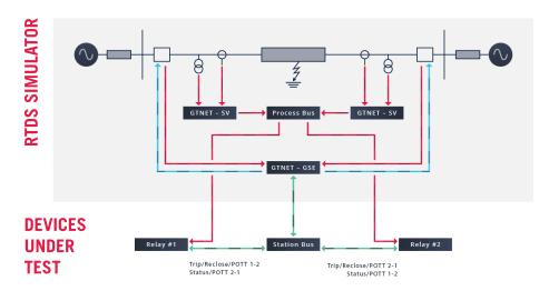
When testing IEC 61850-compliant devices, the secondary voltage and current signals can be provided to the protection equipment via a GTNETx2 card running the GTNET-SV protocol.
