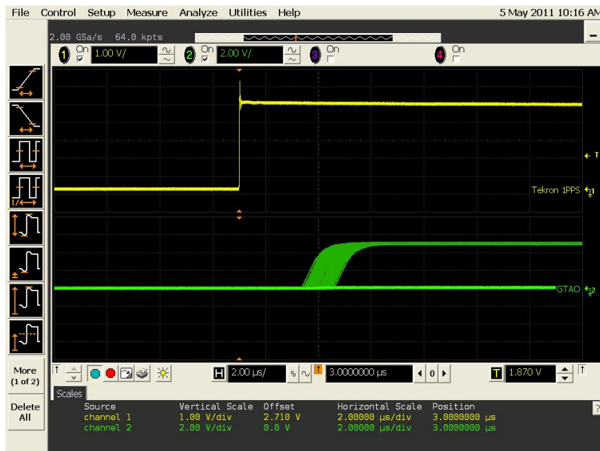
Figure 1: Oscilloscope capture showing analogue output jitter less than \pm 1 \mu s vs 1PPS signal
