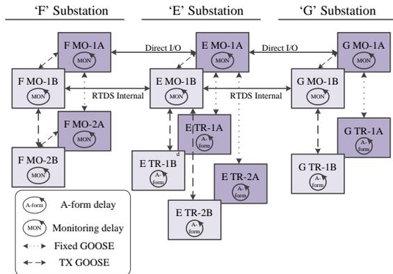
**Figure 4: Major Delays in RAS Processing and Communication**
