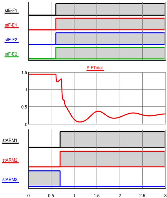
**Figure 7: Contingency Transient (Top to Bottom): E-F Line Breakers, Total Power Flow on the Three Lines Normalized to the F-G Rating, and the Arming During Transient**
