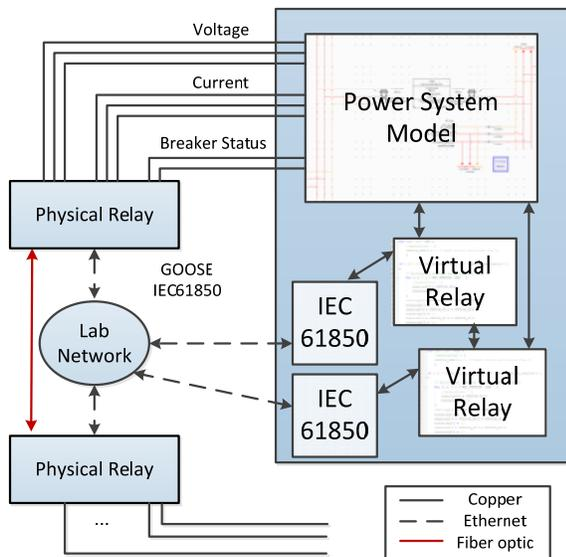
**Figure 3: Lab test setup**
