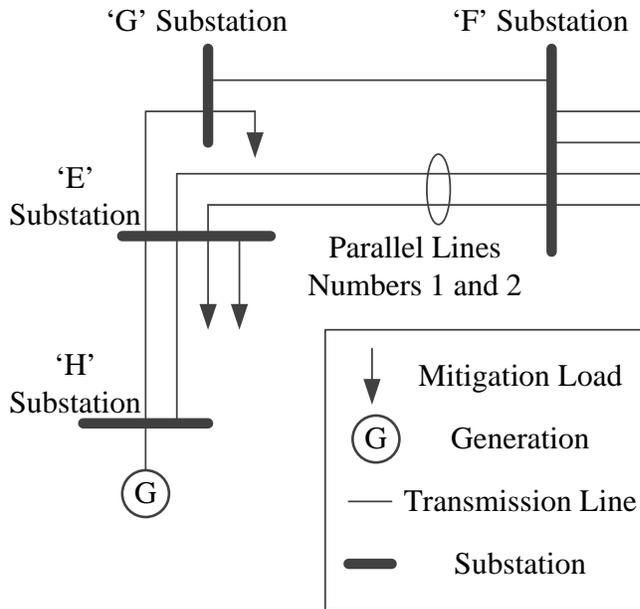
**Figure 2: Diagram of the RAS Local Power System**
