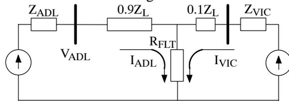
Figure 4: Equivalent Fault Circuit
