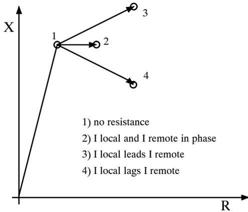
Figure 5: Impact of local and remote fault current on apparent impedance for resistive faults
