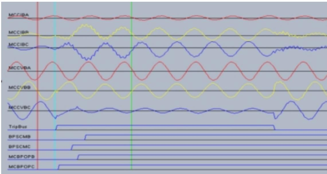
Figure 6: Waveforms obtained from Simulation of a Fault behind Series Capacitor
