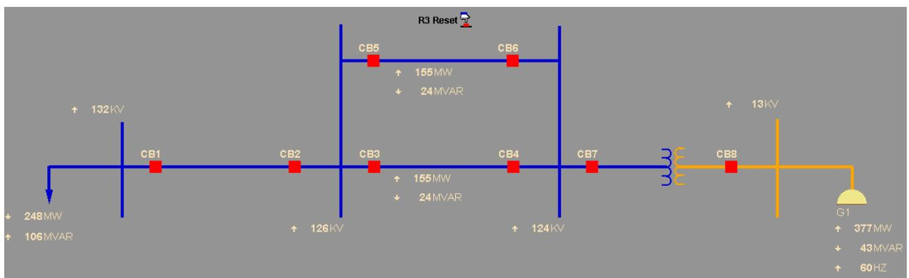
Figure 7. SCADA Display at SNL: Corrupted SCADA Data
