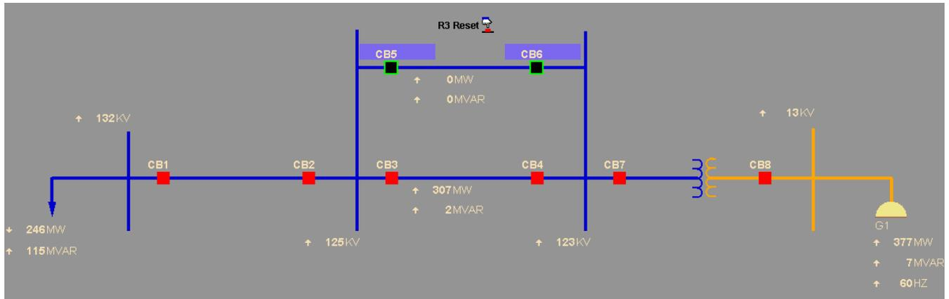
Figure 6. SCADA Display at CAPS: Correct SCADA Data
