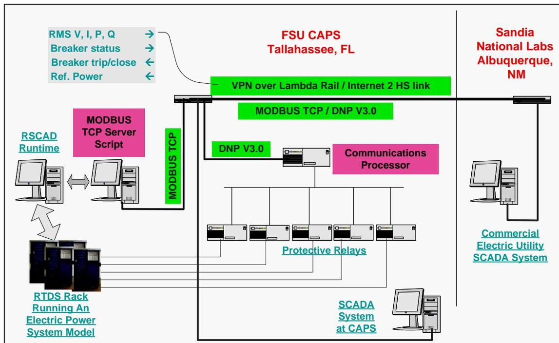
**Figure 4. Diagrammatic Representation of CAPS-SNL Power System Security Testbed**
