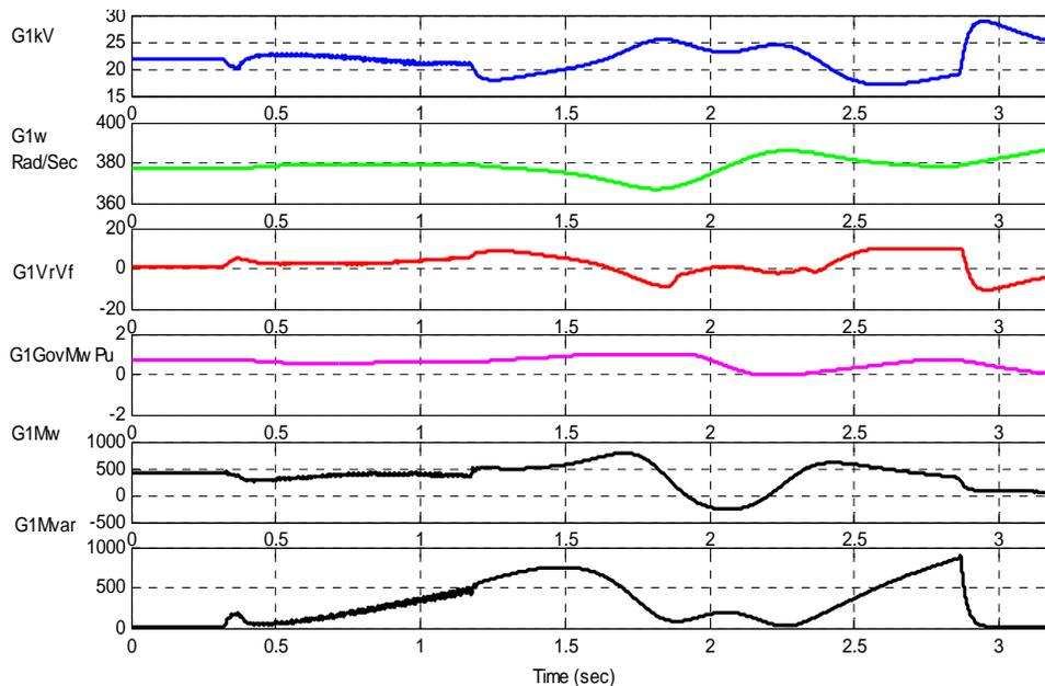
**Figure 9. Generator Terminal Voltage (G1kV), Speed (G1W), Regulator Output (G1VrVf), Governor Output (G1GovMuPu), Active Power (G1Mw) and Reactive**
