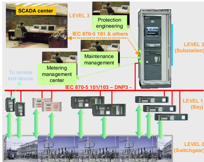
**Figure 2. Typical modern substation showing apparatus and communication links**
