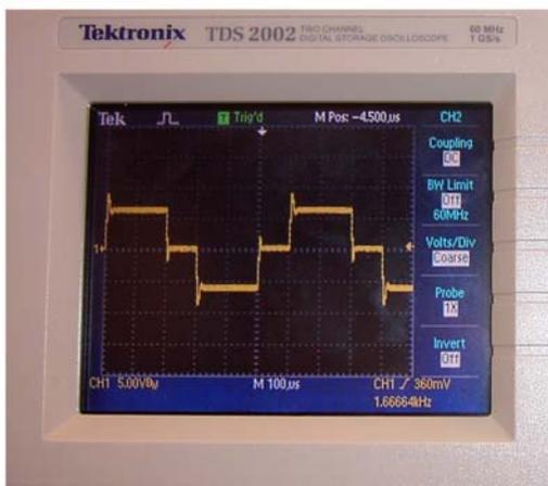
Fig. 4. Three-Level Bridge Voltage Waveform
