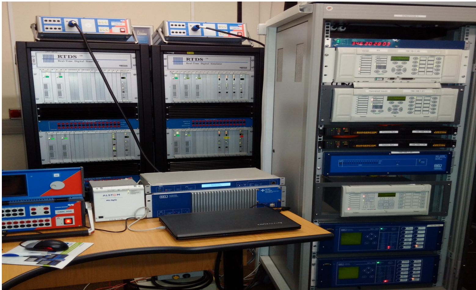
Figure 4: Implemented WAMPAC testbed
