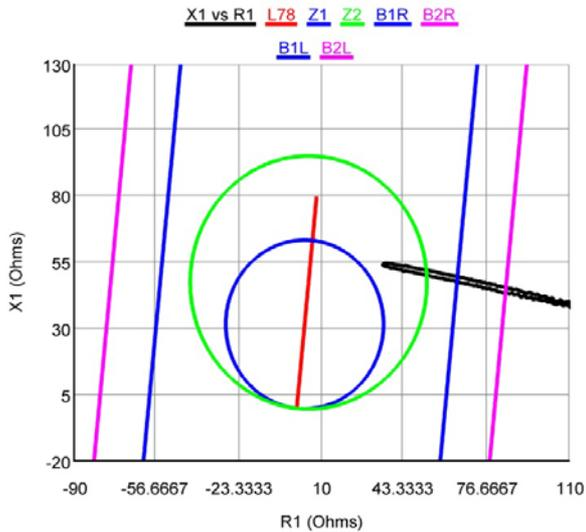
Impedance locus for external fault and stable swing.
