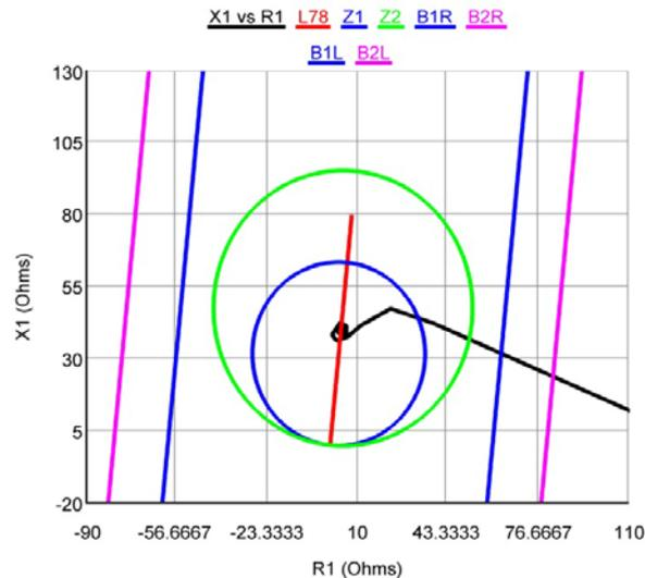
Impedance locus for internal fault.
