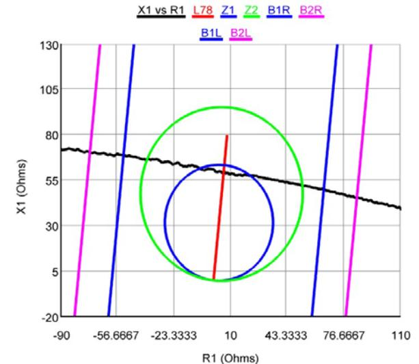
Impedance locus for external fault and unstable swing.
