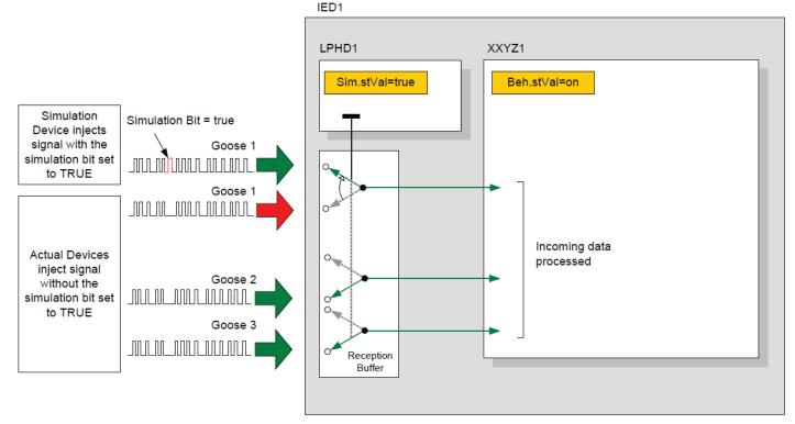
**Example of an IED (IED1) receiving simultaneously simulation and actual signals** -To allow the IED1 to process the simulated Goose1 message instead of the actual Goose 1 message, the Data Attribute Sim.stVal in the LN LPHD1 shall be set to TRUE
