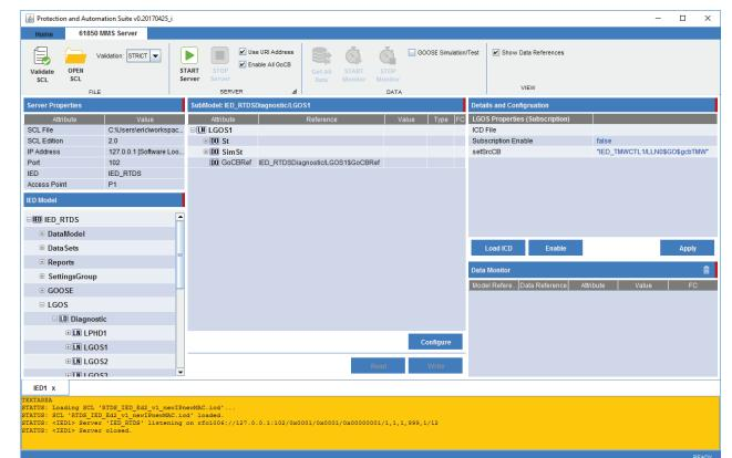
\*Logical Node LGOS allows a subscriber to either subscribe not simulated GOOSE telegrams or simulated GOOSE telegrams
