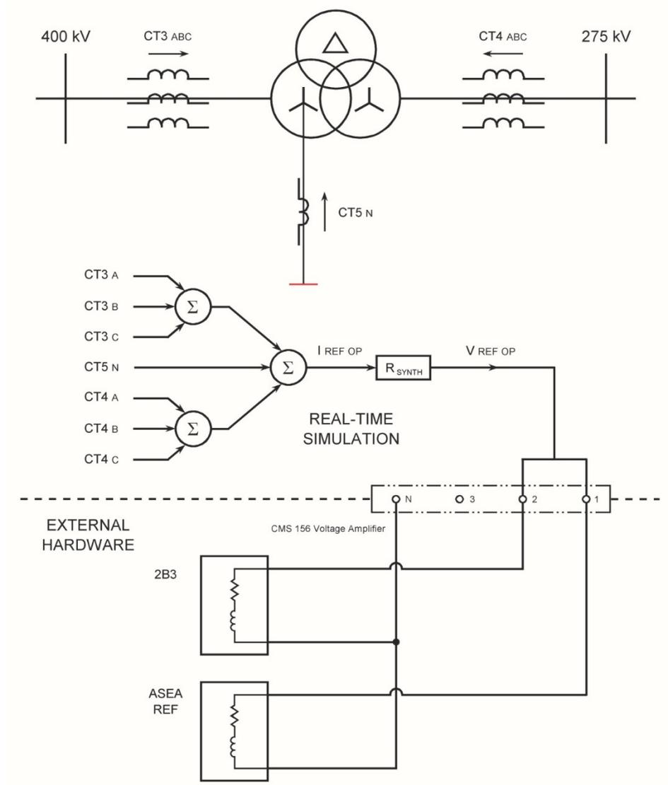
Improved CT models suitable for restricted earth fault relay testing?
