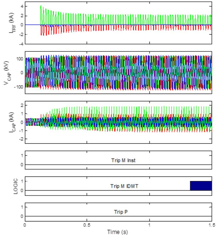
Electronic Relay (MCGG) trips on IDMT O/C
