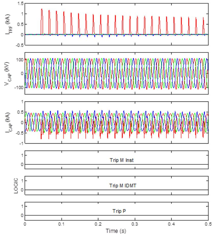
**Both Electronic Relay (MCGG) and Numerical Relay (P122) stable in this case**
