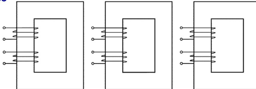
Three separate (uncoupled) cores (a common assumption in simulation models of three-phase transformers).
