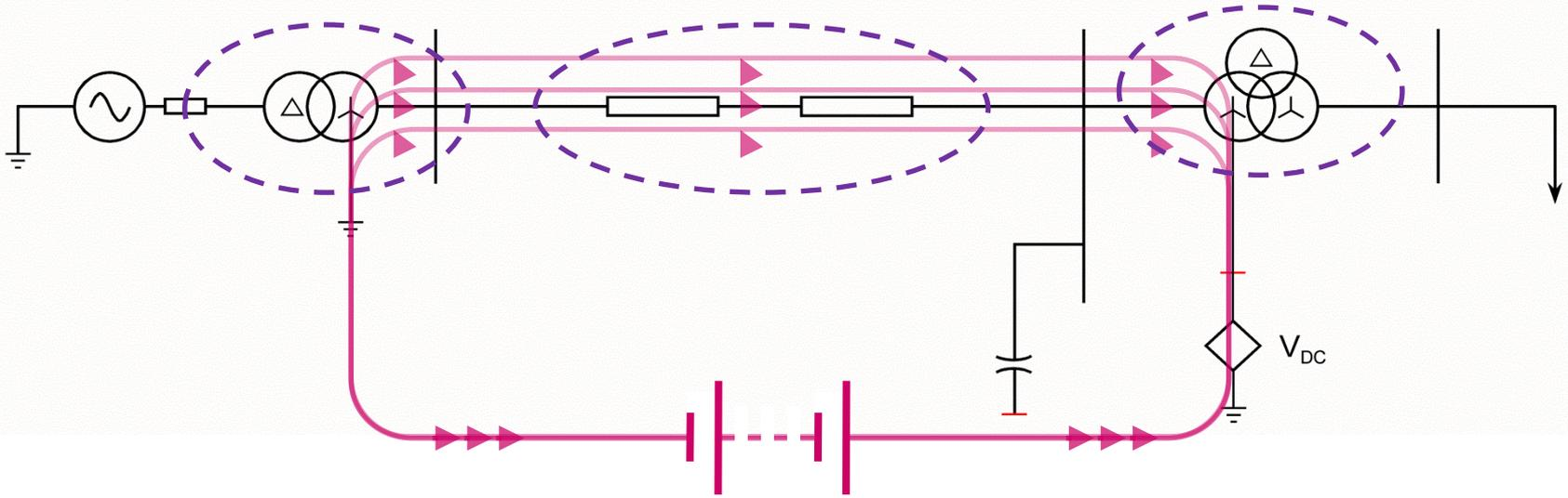
Transmission lines in such studies must therefore be represented using frequency-dependent models capable of correctly describing their impedances in the frequency range between DC and several multiples of 50 Hz.
