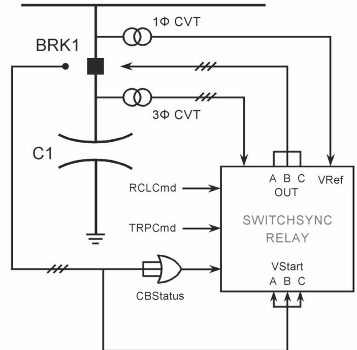
Three binary outputs (**OUT A, B, C**) to close each pole of the breaker.
