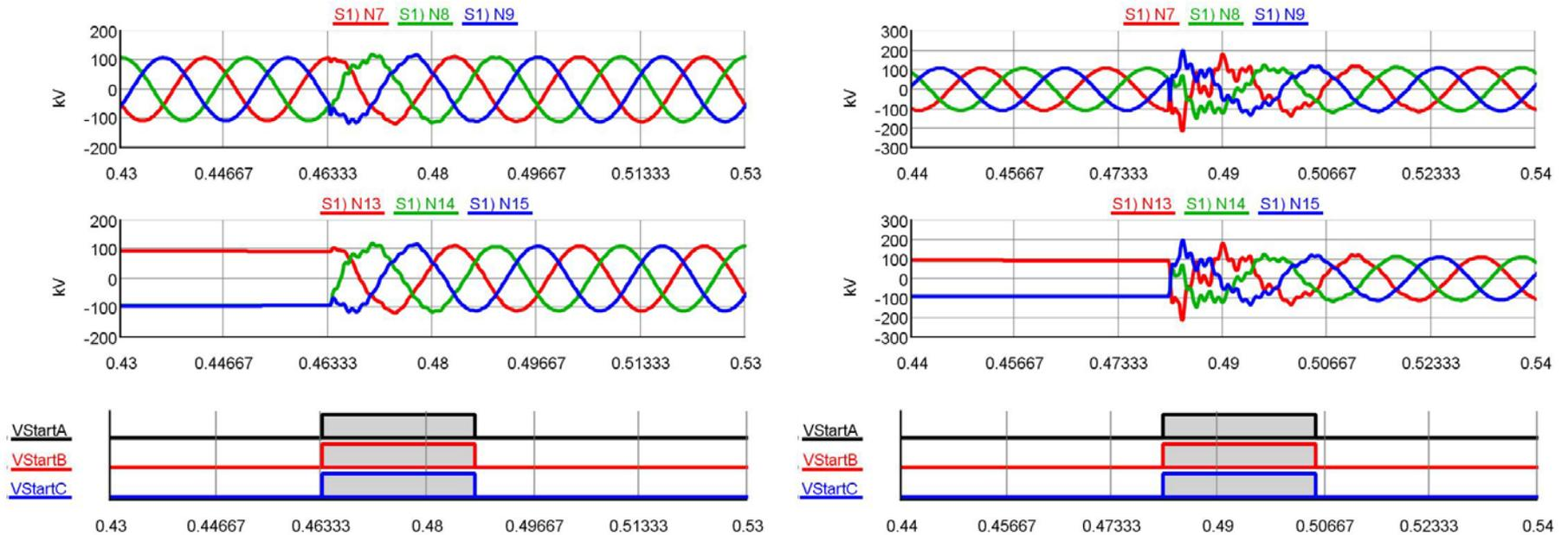
Fig. 2 – All-simulation reference study: capacitor bank reconnected with maximum trapped voltages on its phases; (a) best point on wave for breaker closing; (b) worst point on wave for breaker closing in phase A.
