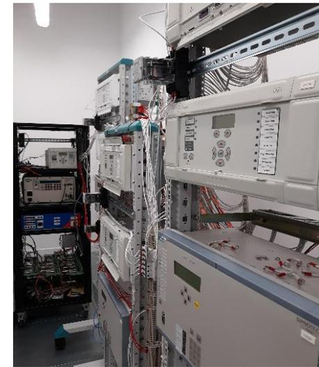
A test setup with Physical relays at our centre
