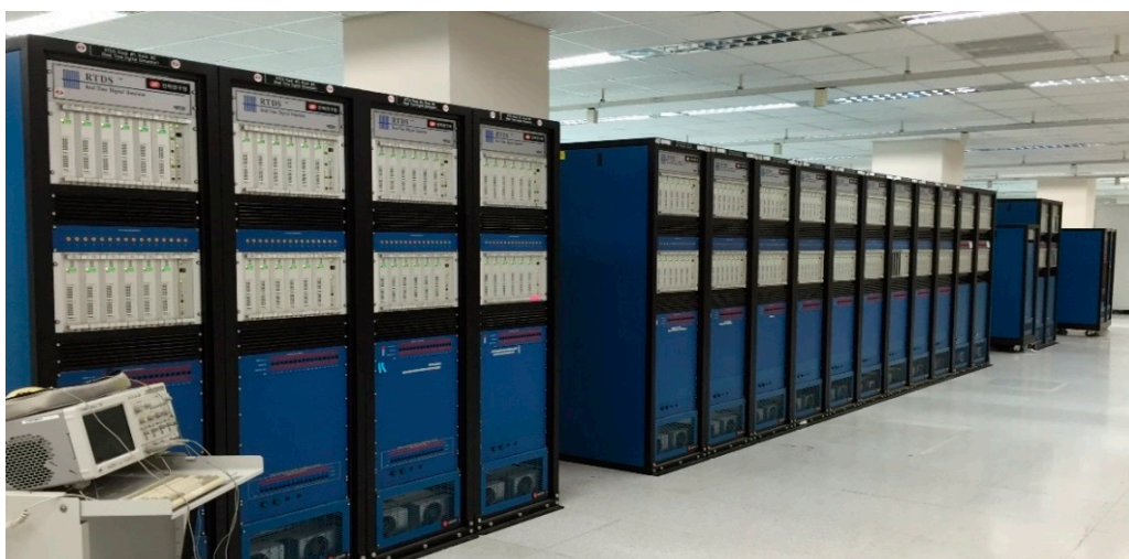
Figure 3. Real-time Digital Simulator in the Korea Electric Power Corporation (KEPCO) Research Institute.
