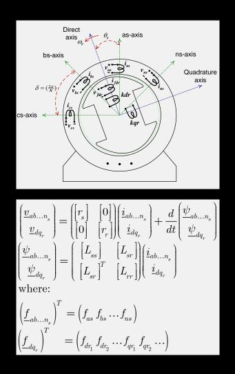
Inclusion of Electric Machine Models into the Network Solution of RTDS
