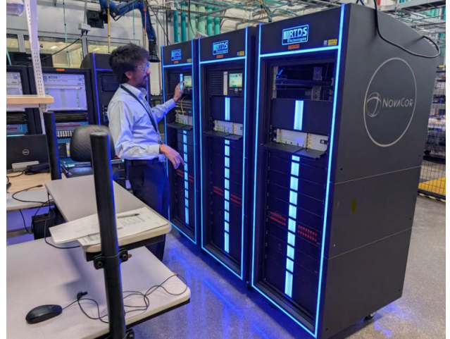
The RTDS Simulator used for data center testing at NLR
