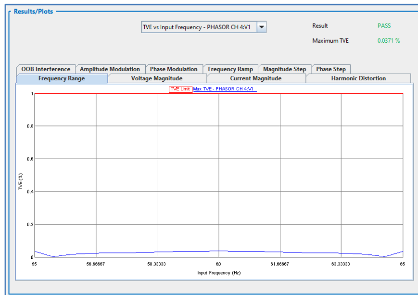
Fig. 7 : TVE Variation of +ve Sequence Voltage under Frequency Range
