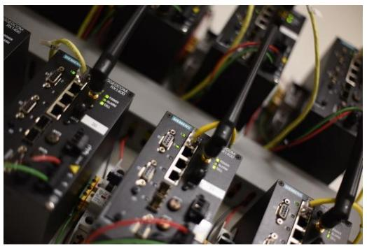
Figure 11 – Communication infrastructure with 23 RX1400 Modems
