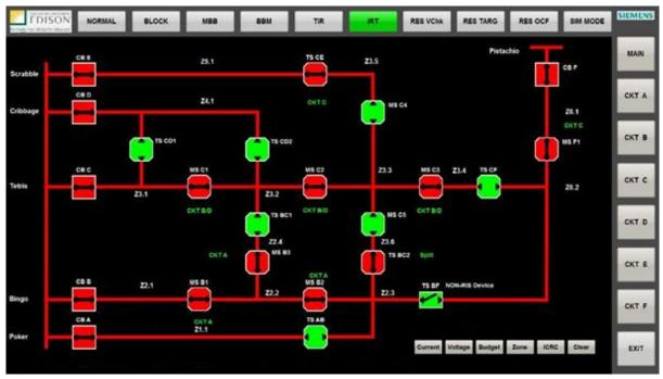
Figure 9 – Main HMI Screen
