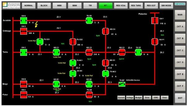
Figure 16 – System response to evolving fault in Zone 5.1
