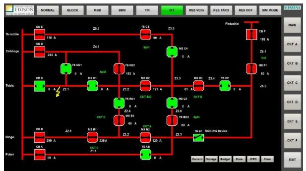
Figure 14 – System response to a fault in Zone 3.1
