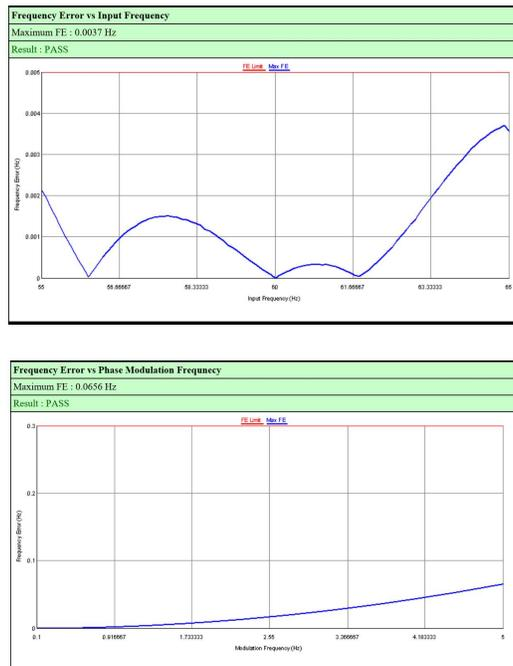
Figure 13: PMU Test Results using RTDS
