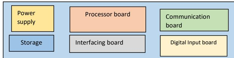
Figure 4: Hardware architecture of the monitoring IED prototype
