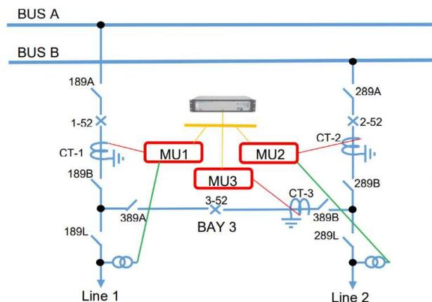
Figure 1: Subscribing data from multiple merging units
