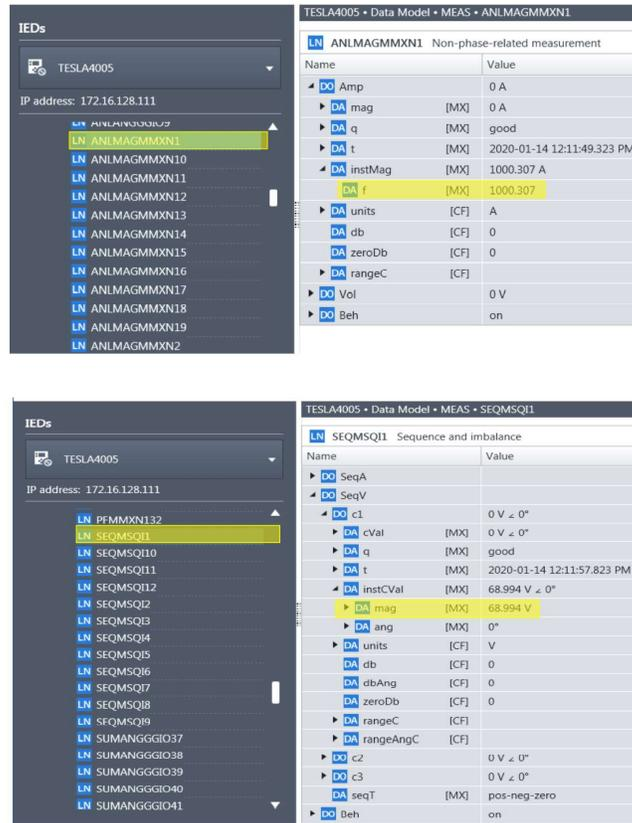
Figure 11: Measurements from IEC 61850 server, including (a) Phase A current, (b) Positive sequence voltage
