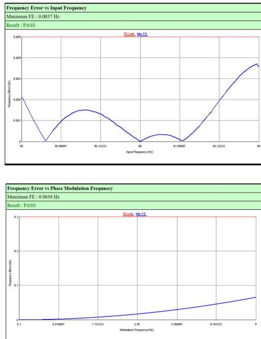
Figure 13: PMU Test Results using RTDS
